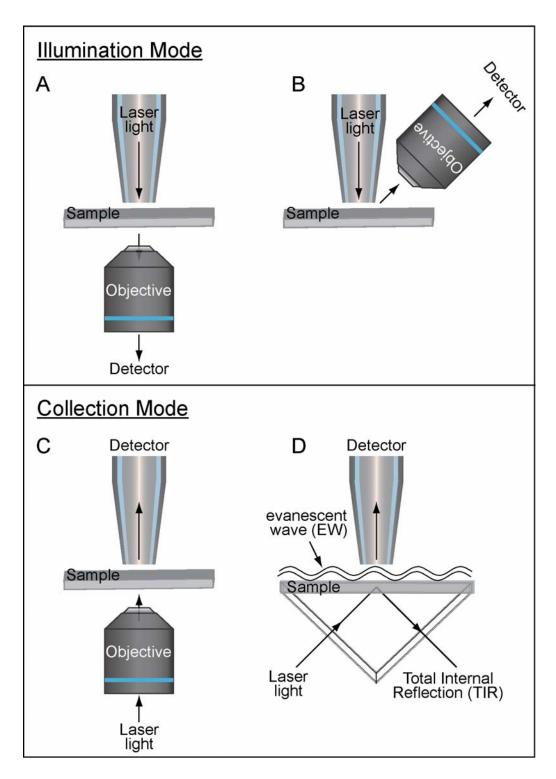
**Figure 2.3.** Scheme of NSOM in (A-B) illumination and (C-D) collection configurations.
