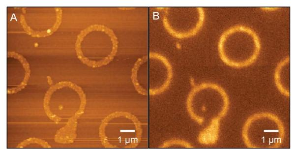
**Figure 2.4.** (A) Topography image of rings of 25-nm high CdSe/ZnS NCs and (B) corresponding fluorescence NSOM image.
