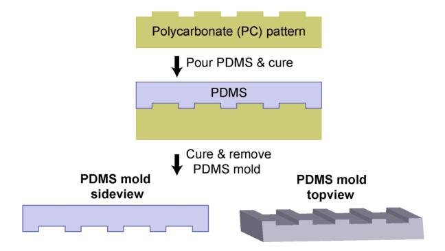
Figure 5.3. Scheme for making PDMS mold using PC layer.
