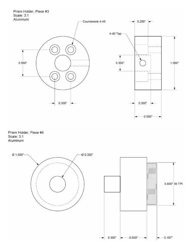
Figure A1.2. CAD drawings of piece 3 and piece 4 of prism holder.
