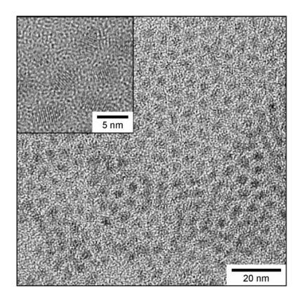
**Figure 3.4.** TEM micrograph of CdSe QDs. Inset : High-resolution TEM micrograph shows the crystalline and slightly oblong nature of the CdSe QDs.
