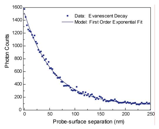
Figure 2.7. Photon counts as a function of increasing distance z from the sample interface. Probe-surface separation was measured from the point at which the probe was in feedback.
