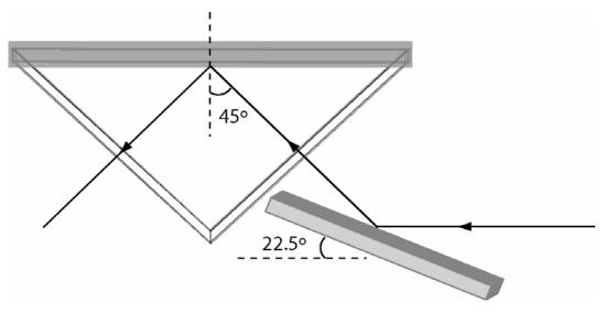
Figure A1.4. Diagram showing the mirror position with respect to the prism.
