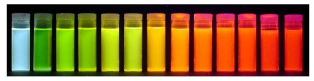
**Figure 3.2.** Fluorescence image of CdSe quantum dots showing an increase in QD size going from blue (~1 nm in diameter) on the left to red (~5 nm in diameter) on the right.
