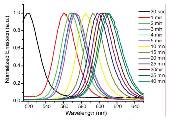
**Figure 3.3.** Emission spectra FWHM of ~30 nm of CdSe QDs in hexanes. Time indicates when the aliquots were taken after injection of the Se-stock. Spectra correspond to the image in Figure 1.
