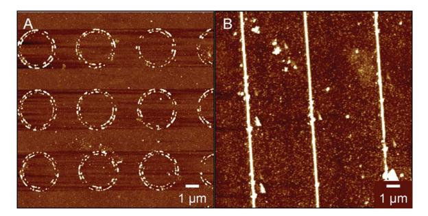
**Figure 3.8.** (A-B) AFM images of quantum dots patterned into rings and lines using the templates from Figure 3.4. Lines with well-packed quantum dots were as narrow as 100 nm, and the height of the quantum dot structures varied between 15-50 nm.
