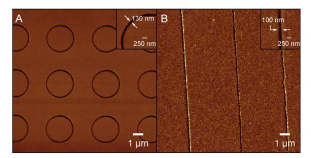
**Figure 3.5.** AFM images of (A) rings and (B) trenches formed in negative tone resist using phase-shifting photolithography. These linewidths can be as narrow as 100 nm.
