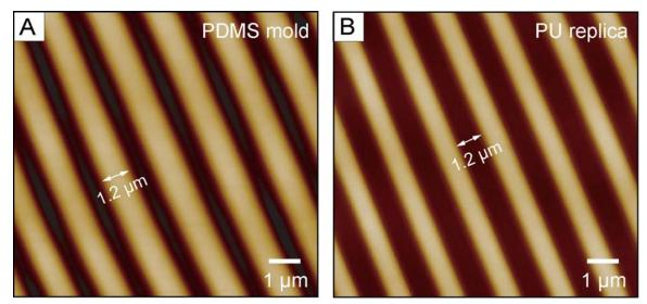
**Figure 5.8.** AFM images of (A) PDMS mold from Al-layer and (B) PU-replica of the Allayer after MIMIC. Dark regions correspond to recessed features, and bright regions correspond to raised features.
