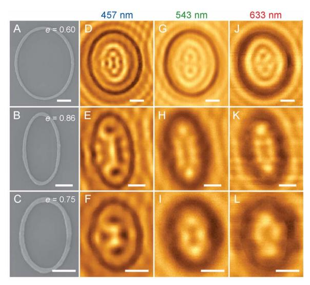
**Figure 4.7.** SEM images of ellipses with eccentricity of (A) 0.60, (B) 0.86, and (C) 0.75 imaged with (D-F) 457-nm, (G-I) 543-nm, and (J-L) 633-nm light. All the optical images were acquired with circularly polarized light. All scale bars are 1  $\mu$ m.
