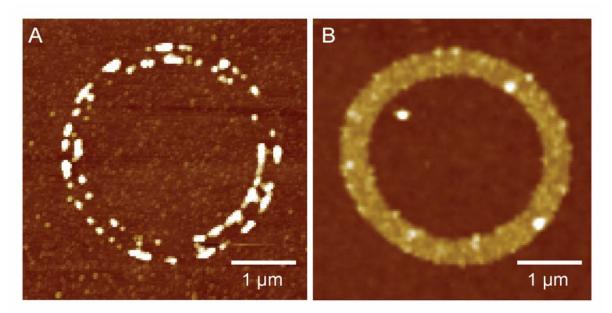
**Figure 3.7.** AFM images of quantum dots assembled into ring templates after (A) 12 hours and (B) two days of sedimentation.
