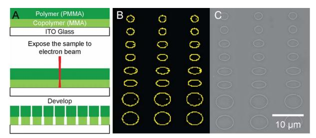
**Figure 2.12.** (A) Schematic illustration of e-beam lithography. (B) DesignCAD drawing of desired patterns, and (C) SEM image of metal ellipses produced after deposition and lift-off of the resist template.
