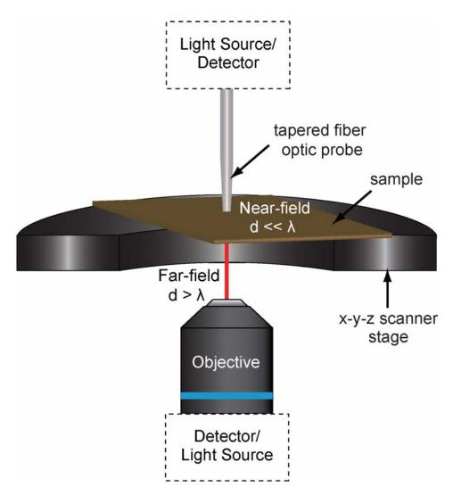
**Figure 2.1.** Schematic diagram of an NSOM configuration. Boxes with dashed lines indicate the components that can have two different positions.
