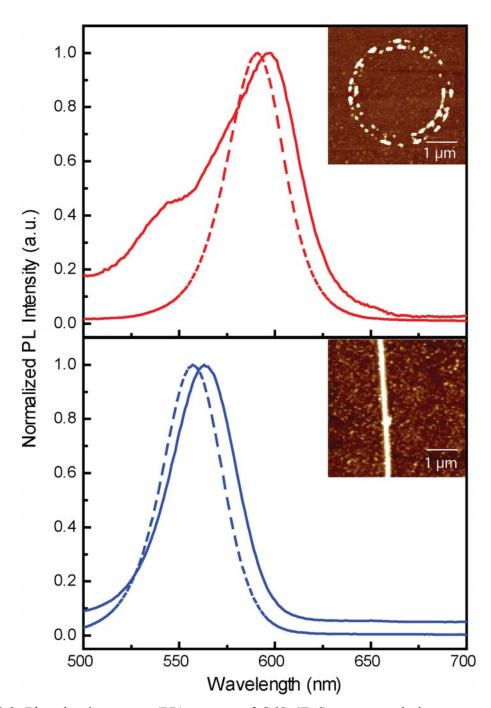
**Figure 3.9.** Photoluminescence (PL) spectra of CdSe/ZnS nanocrystals in aqueous solutions (dashed lines) and patterned on substrates (solid lines) from Figure 3.6. Both (A) larger dots patterned into rings and (B) smaller dots patterned into lines exhibited a red-shift in the PL compared to the same dots in dilute solutions. The insets represent the mesoscale patterns of the CdSe/ZnS dots from which the PL was measured.
