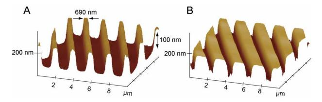
**Figure 5.6.** AFM images of (A) PDMS mold from PC layer and (B) polyurethane replica of PC layer formed by curing PU against the mold in (A).
