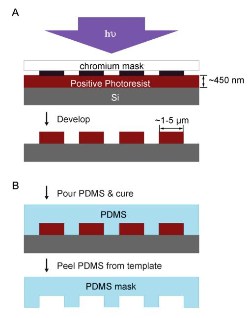
**Figure 2.10.** Schematic illustrations of the (A) fabrication of photoresist masters and (B) fabrication of PDMS mask.
