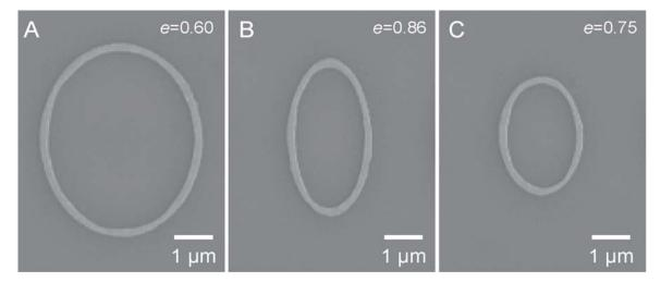
**Figure 4.2.** SEM image of Au ellipses with eccentricities (*e*) of (A) 0.60, (B) 0.86, and (C) 0.75.
