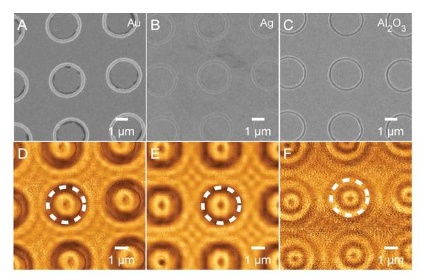
**Figure 4.6.** SEM images of (A) Au, (B) Ag, and (C) Al<sub>2</sub>O<sub>3</sub> rings on ITO/glass and their corresponding collection mode NSOM images (D-F). White dashed rings on the NSOM images indicate the position of the ring structures.
