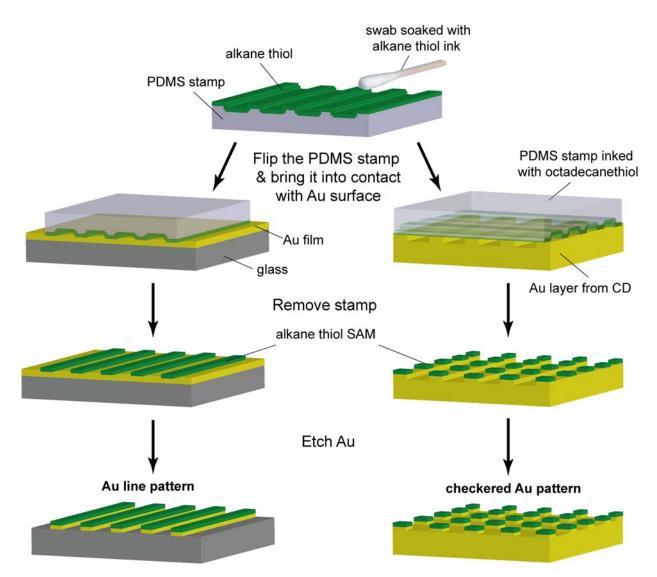
**Figure 5.9.** Procedure for micro-contact printing and etching of a Au film (left) and a Au-CD (right).
