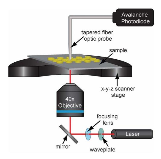
Figure 4.3. Scheme of collection mode NSOM set-up used for imaging the corrals.
