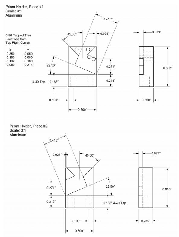
Figure A1.1. CAD drawings of piece 1 and piece 2 of prism holder.
