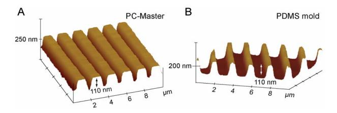
Figure 5.4. AFM image of (A) PC-master and (B) PDMS mold formed from (A).
