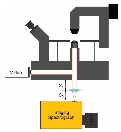
Figure 2.8. Microscope-spectrometer set-up for single particle spectroscopy.
