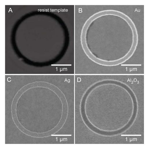
Figure 4.1. AFM image of (A) photoresist template for circular corrals and SEM images of (B) Au, (C) Ag, and (D)  $Al_2O_3$  rings on ITO/glass substrate.
