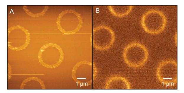
**Figure 3.10.** (A) Topography image of rings of 25 nm high CdSe/ZnS dots and (B) corresponding fluorescence NSOM image of arrays of quantum dots patterned into ring structures.
