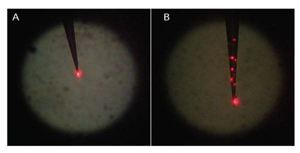
**Figure 2.2.** Optical micrograph of pulled NSOM probes (A) without and (B) with pinholes.
