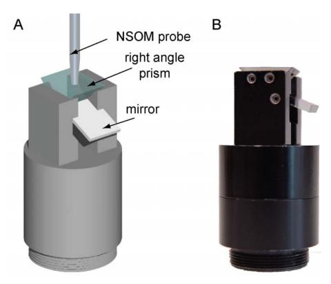
**Figure 2.6.** (A) Scheme and (B) optical micrograph of prism holder for PSTM set-up.
