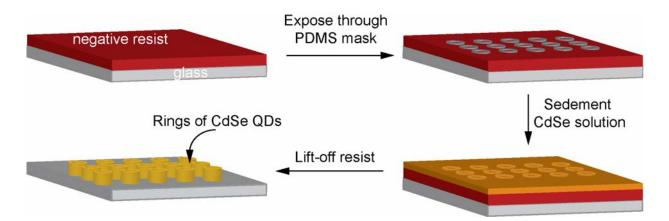
**Figure 3.6.** Schematic illustration for patterning chemically synthesized nanomaterials using templates made of photoresist. A pattern is produced in negative-tone resist using PSP with composite PDMS masks. The scheme depicts an example of a ring generated by PSP using a mask patterned with circular, recessed posts. The nanomaterials assembled into the recessed regions of the template by sedimentation. Removal of the photoresist generated arrays of structures in specific patterns.
