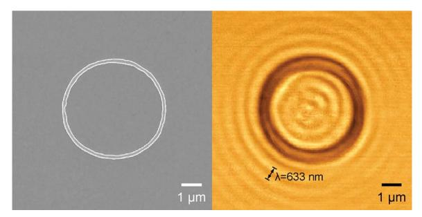
**Figure 4.4.** SEM image of (A) 4.8-µm Au ring and (B) corresponding optical NSOM taken with circularly polarized 633-nm light.
