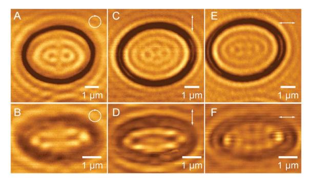
**Figure 4.8.** Ellipses with *e* of 0.6 and 0.86 imaged using 543-nm light with (A-B) circular polarization, (C-D) linear polarization along the long axis, and (E-F) linear polarization along the short axis.
