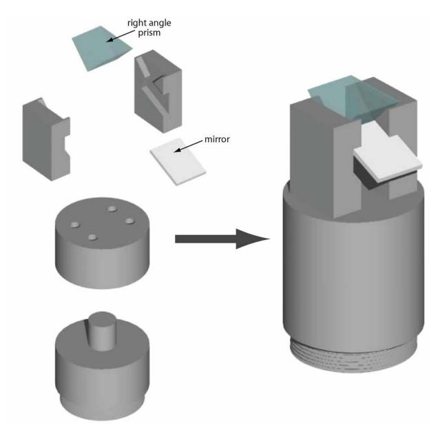
Figure A1.3. Components of prism holder.
