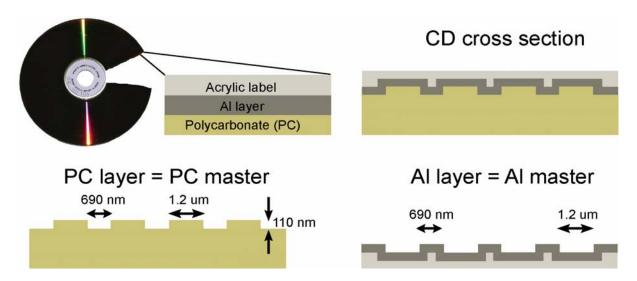
Figure 5.1. Cross section of a CD.
