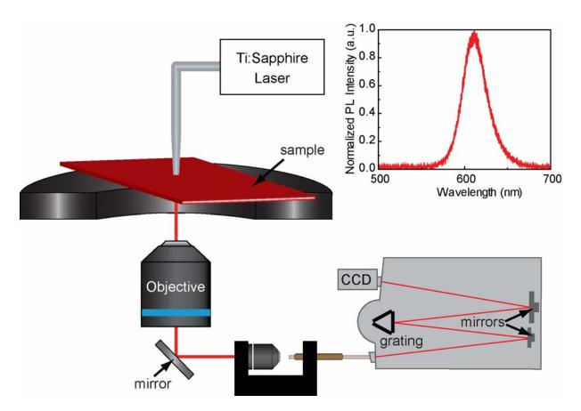
**Figure 2.5.** Scheme of transmission NSOM coupled with a spectrometer. Inset: photoluminescence spectra from water soluble CdSe/ZnS QDs drop-coated onto a glass slide.
