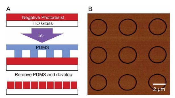
**Figure 2.11.** (A) Schematic illustration of PSP and (B) AFM image of recessed rings in negative tone resist produced by PSP.
