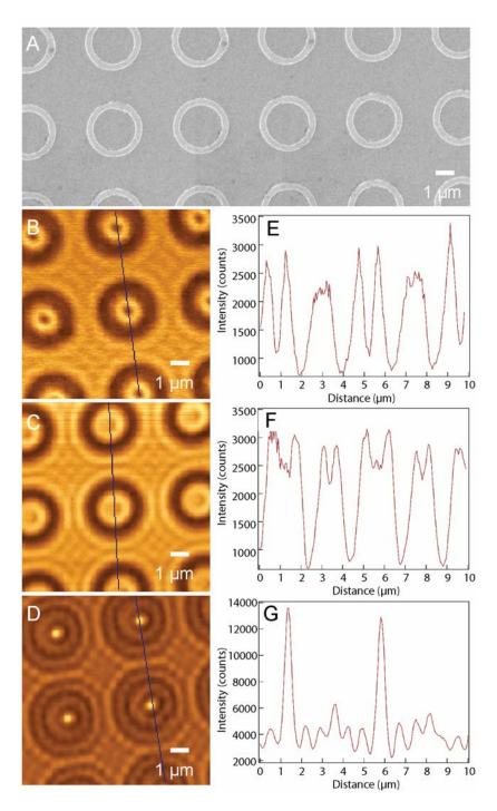
**Figure 4.5.** (A) SEM image arrays of 2.35-µm Au rings. Collection mode NSOM images of 3-µm rings imaged with (B) 633 nm, (C) 543 nm, (C) 457 nm light and their corresponding cross sections (E-G).
