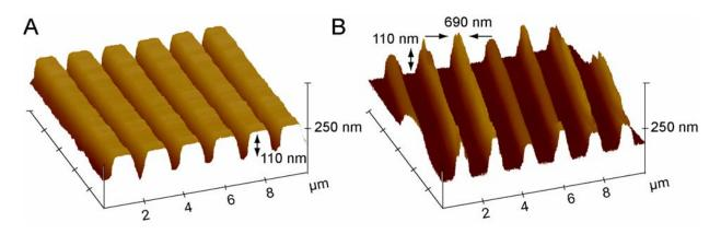
Figure 5.2. AFM images of (A) PC layer and (B) Al layer obtained from a CD-R.
