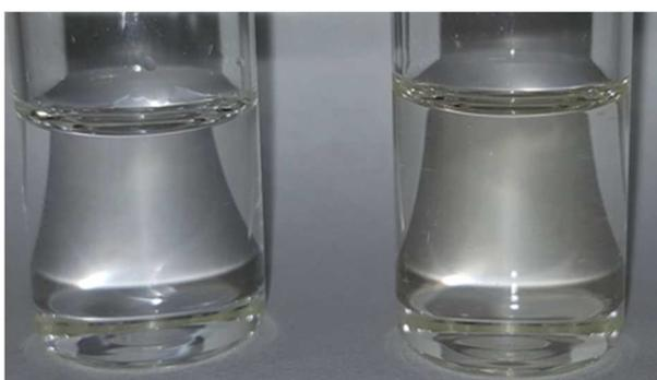
Figure 8: Vial of pure PAO4 (left) and a 5 wt % solution of the in PAO4 (right), which shows a yellow tint and no insoluble material.
