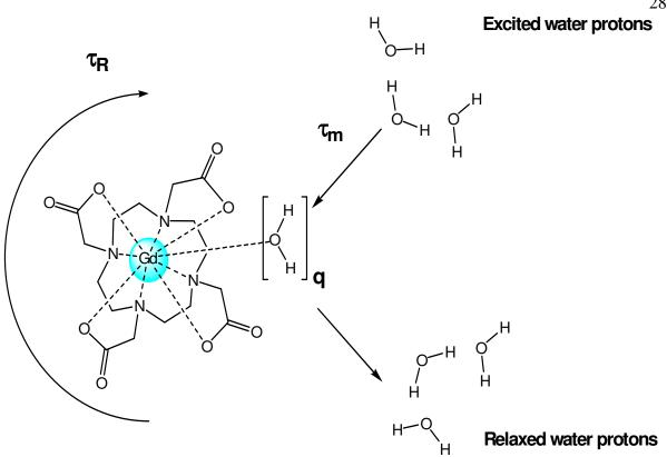
**Figure 1.2.** Factors affecting relaxivity of Gd(III)-based MR contrast agents: the hydration number (*q*), the mean residence lifetime of bound water molecules ( $\tau_m$ ), and the rotational correlation time ( $\tau_R$ ).
