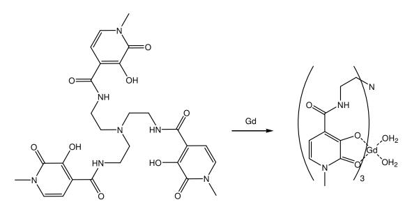
**Figure 1.3.** Structure of Gd-TREN-1-Me-3,2-HOPO, a q = 2 contrast agent.<sup>12</sup>
