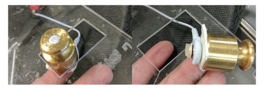
Figure 4.7. Conditions at the fingertip for measuring the bioimpedance of the skin and body. The small Ag/AgCl electrode was stamped out from a larger electrode, and attached to a weight, which was then allowed to bear against the finger. An acrylic frame constrained the weight horizontally.
