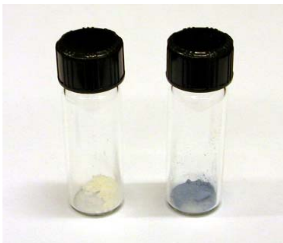
Figure 2.4 A) Color change of 4 (left) upon exposure to lithium naphthalenide (right). B) Color change of 2 (left) upon exposure to lithium naphthalenide (right).
