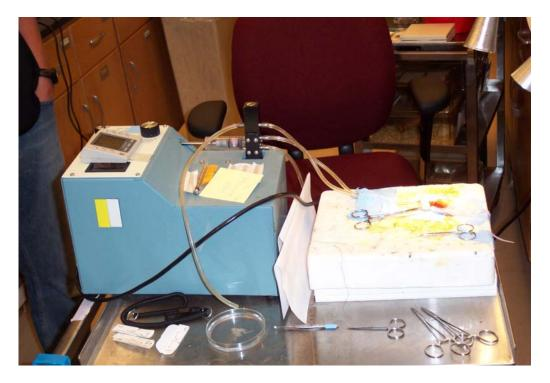
Figure 28: Ventilator used for intubating anesthetized mice.
