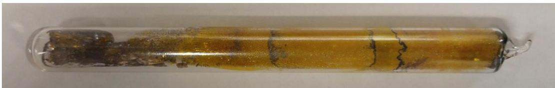
**Figure 118.** Vapor Transport tube after the transport experiment shows the transported  $\text{PbI}_2$  on the right side of the image. The black solid on the left hand side is the remaining  $\text{AuPb}_2\text{I}_7$  grown on  $\text{PbI}_2$ , with a dominant amount of metallic gold. This was in the hot zone.
