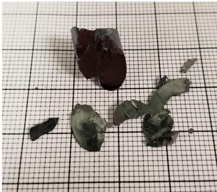
**Figure 19.** A representative ingot of  $(\text{PbI}_2)_{0.5}(\text{BiI}_3)_{0.5}$  after the molten mixture is slowly cooled. Large crystalline regions can be cleaved from these samples for charge transport measurements.
