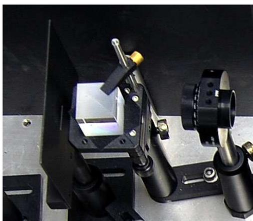
**Figure 6-5: PBS cube, Mask, and Half-wave Plate**
