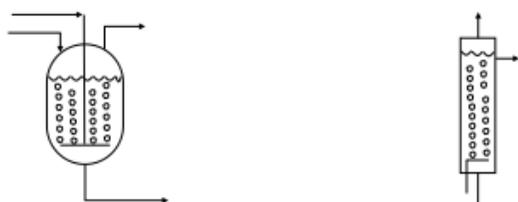
Figure 11. Sparged stirred tank and tubular reactors (Towler, 2012)
