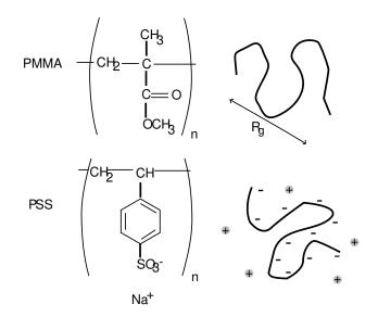
Figure 2.1. Illustration of Polymethyl methacrylate (PMMA) and Sodium polystyrene sulfonate (PSS) showing the chemical structure of the repeat unit. The physics point of view considers a polymer as a gaussian chain, with radius of gyration,  $R_g$ . The polymer is considered to have a uniform line charge, with counterions in solution.
