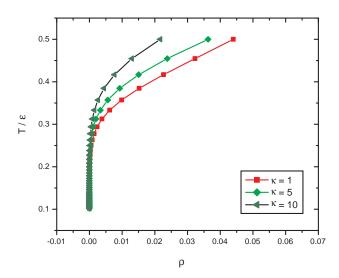
Figure 7.8. Phase diagram of for a symmetric 1:1 mixture for increasing values of  $\kappa$ , inverse screening length. Increasing  $\kappa$  requires lower values of short range interactions,  $\varepsilon/T$ , for phase coexistence. The solid phase has constant density  $\rho_{solid}$ .
