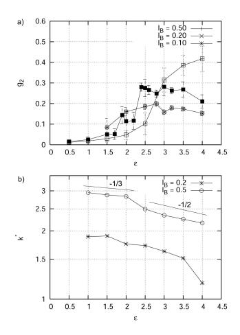
Figure 5.6. a) The interfacial orientational order parameter  $g_2$  at several values of the Bjerrum length  $(l_B = 0.1\sigma, 0.2\sigma, 0.5\sigma)$  as a function of  $\varepsilon$ . As the orientational order of the domains increases,  $g_2$  increases from 0 to a finite value. b) The location of the peak  $k^*$  in the structure factor  $S(\vec{k})$  as a function of  $\epsilon$ . The scaling of  $k^*$  with  $\varepsilon$  changes from -1/3 to -1/2.
