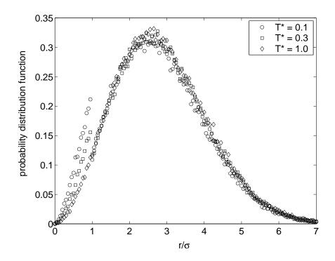
Figure 3.6. The probability of the chain end-to-end distances r in units of the width of the square potential  $\sigma$  at a reduced density  $\rho^* = 0.05$  for different effective temperatures  $T^* = 0.1, 0.3, 1.0$ . For all values of  $r/\sigma > 1$  the probability is Gaussian and it is independent of  $T^*$ . Deviations from the Gaussian distribution are observed at length scales smaller than  $\sigma$  when  $T^*$  is very low.
