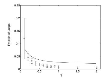
Figure 3.9. Fraction of chains that belong to loops as a function of reduced temperature  $T^*$  at several a reduced density of 0.15 ( $\rho^* = 0.15$ ). The theoretical results are marked with a solid line, while the simulation results are represented by circular points. Standard deviation is indicated. Disagreement is seen with theoretical results at both low and high temperatures.
