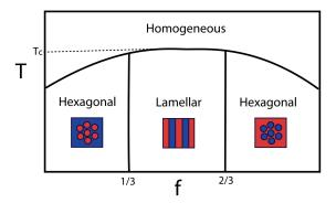
Figure 8.1. Phase diagram of the minimum free energy as a function of charge fraction, f, and temperature, T. At high temperatures the density is homogeneous. As temperature is decreased there is a transition temperature,  $T_c$ , at which a periodic phase forms. For charge fractions, 1/3 < f < 2/3, the minimum free energy phase is lamellar. Outside this region the minimum free energy is hexagonal. Figure adapted from Solis et al.
