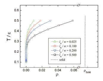
Figure 7.6. Phase diagram of the mixture. Location of solid-gas coexistence curves in  $\rho - T$  plane is shown for several different values of the Bjerrum length,  $l_B/\sigma$ . Increasing the Bjerrum length requires higher values of short range interactions,  $\varepsilon/T$ , for phase coexistence. The solid phase has constant density  $\rho_{solid}$ . The figure refers to the case of equal charge density  $z_+/z_- = 1$ , which forms a lamellar microphase.
