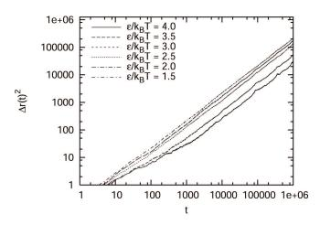
Figure 5.11. Mean square displacement as a function of timestep at  $l_B/\sigma = 0.5$  for values of  $\varepsilon/k_BT = 1.5 - 4.0$ . While diffusion is linear initially, nonlinearity starts developing at  $\varepsilon/k_BT = 4.0$
