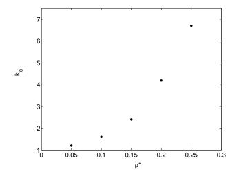
Figure 3.11. Values of  $k_o$  obtained from numeric fits to thermodynamic results obtained from simulation at several densities. As the density is increased, the value of  $k_o$  also increases.
