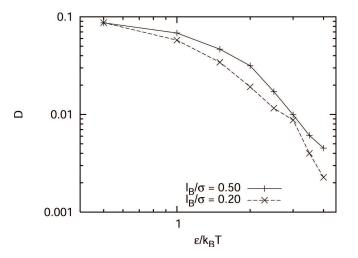
Figure 5.2. Diffusion coefficient, D, as a function of short range interaction  $\varepsilon/k_BT$ , for two comparable values of the Bjerrum length,  $l_B/\sigma = 0.2, 0.5$ . With increasing  $\varepsilon$ , faster diffusion is seen for higher values of  $l_B$ , but both systems approach a regime of very small diffusion.
