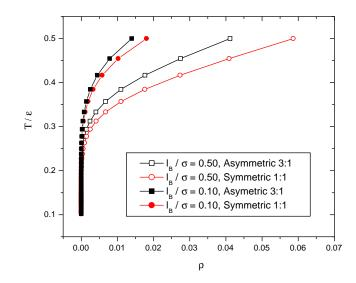
Figure 7.7. Phase diagram of asymmetric 3:1 and symmetric 1:1 mixtures for two different Bjerrum lengths. Increasing the asymmetry of the mixture requires lower values of short range interactions,  $\varepsilon/T$ , for phase coexistence. The solid phase has constant density  $\rho_{solid}$ .
