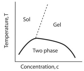
Figure 3.1. Schematic phase diagram for a polymer gel versus temperature and concentration.
