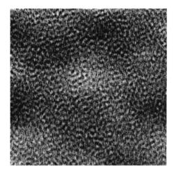
Figure 4.1. AFM images of absorbed surfactant micelles on silica at 25C.  $300nm \times 300nm$ . Reproduced from Ducker et al [88].
