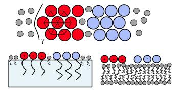
Figure 7.3. Schematic of neutral and charged components strongly adsorbed to a liquid interface, such as an emulsion or the surface of a bilayer. The charged components segregate into a periodic solid phase with line tension  $\gamma$  within a homogeneous background.
