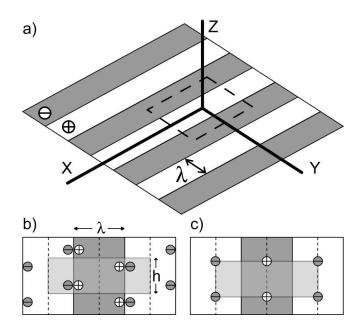
Figure 6.7. a) The schematic representation of the system. The basic Wigner lattices formed by condensed b) ions forming dipoles and c) single ions.
