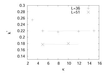
Figure 6.6. The location of the peak,  $k^*$ , in the structure factor, S(k), as a function of  $\kappa$  from simulation results spanning a range of the screening parameter ( $\kappa = 3 - 15\sigma$ ) at an intermediate value of short range attraction ( $\epsilon = 2.0$ ). Increasing the size of the system from L = 36 to L = 51 decreases the average value of  $k^*$ .
