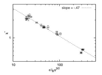
Figure 7.12. The location of the peak  $k^*$  in the structure factor  $S(\vec{k})$  as a function of  $\varepsilon/(l_B\psi^{3/2})$ . The linear fit shows agreement with the scaling predicted by strong segregation theory of power -0.5.
