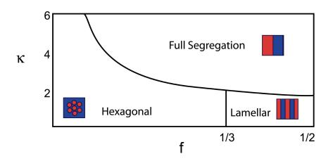
Figure 6.2. For an increase in the inverse screening length,  $\kappa$ , the system jumps from a periodic phase to a fully segregated mixture of opposite charges. Reproduced from Solis et al [118].
