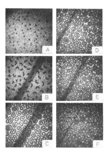
Figure 4.2. Fluorescence micrographs of a 5 mol film at pH 11 and 10 C as upon compression of langmuir monolayer. A) indicates the start of the transition. F) indicates the completion. The lighter regions represent a fluid mixed neutral and charged phase and the darker regions indicate a dense charged region. Reproduced from Heckl et al.[93]
