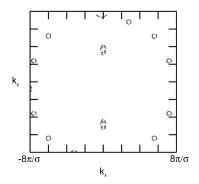
Figure 5.5. Contour plot displaying the location of the peak,  $k^*$ , in the structure factor, S(k), for several values of short range attraction  $\varepsilon = 4.0$  and  $l_B = 0.5$ . The peaks are located at 90 degrees and 270 degrees respectively.
