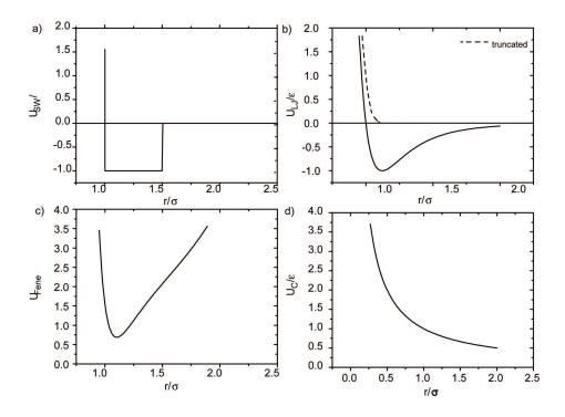
Figure 2.3. Common intermolecular potentials for coarse-grained simulation. a) Square well potential. b) Lennard Jones 6-12 potential. Dashed line represents the truncated and shifted version, including only the repulsive portion of the potential. c) Fene potential d) Repulsive 1/r Coulomb potential.
