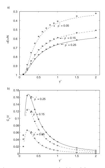
Figure 3.5. Average energy per particle (a) and heat capacity per volume (b) as functions of reduced temperature  $T^*$  at reduced densities  $\rho^* = 0.05, 0.15, 0.25$  with the theoretical results respectively marked with dashed, dot-dashed, and solid lines and the simulation results represented by circular points. Standard deviation is smaller than the width of the circular point, otherwise it is marked.
