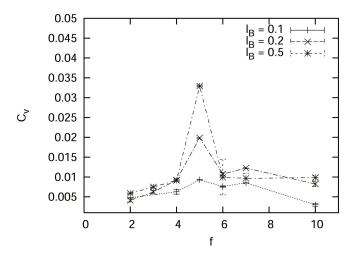
Figure 5.15. Heat capacity per particle as a function of the charge ratio of the components. Fluctuations peak for charge ratios of 5:1. This is the onset of the formation of a Wigner crystalline phase.
