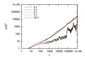
Figure 5.16. Mean square displacement as a function of timestep at  $l_B/\sigma = 0.5$ and  $\varepsilon/k_BT = 4.0$ , for increasing charge ratios of the components. For charge ratios > 5:1, diffusion becomes non-linear. This indicates the formation of a glass.
