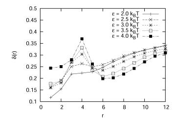
Figure 5.10. Normalized root mean square displacement,  $\delta(r)$ , of the center of masses of domains for increasing values of  $\varepsilon$ . Lindemann Criterion,  $\delta(r)$ , indicates that the local structure of the domains are liquid for these values of the parameters,  $l_B$  and  $\varepsilon$ .
