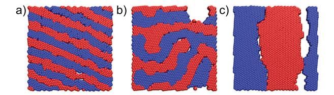
Figure 6.4. Snapshots of the system for  $\epsilon = 4.0$  and  $l_B = .5$ , showing progressive values of screening. a)  $\kappa = 0.2\sigma^{-1}$  b)  $0.4\sigma^{-1}$  c)  $1.0\sigma^{-1}$ . The system melts when  $1/\kappa \sim L$  where L is the width of the periodic domain.
