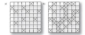
Figure 3.2. a) In the percolation model, each site has a probability, p, of being occupied. An occupied site is denoted by an x. b) When a cluster reaches across the dimensions of the lattice, percolation has occurred.
