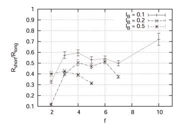
Figure 5.13. Ratio of the asymmetry of the domains as a function of the charge ratio of the components. The most spherical domains are present for charge ratios, f, close to 3:1, while for increasingly asymmetric mixtures, there is a gradual increase in the asymmetry of the domains.
