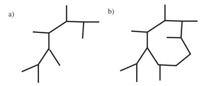
Figure 3.3. a) An illustration of a tree-like structure within classical gelation theory. b) An illustration of a loop-like structure that would not be included in classical gelation theory.
