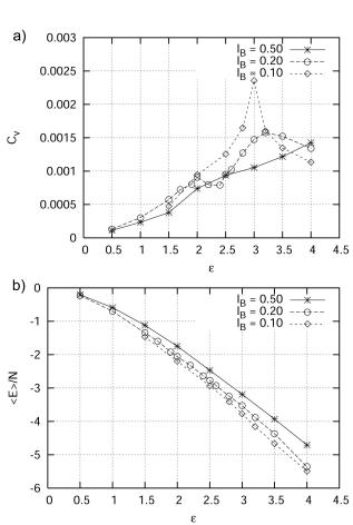
Figure 5.4. a) Heat capacity per particle  $(C_V)$  and b) average internal energy  $(\langle E \rangle /N)$  at several values of the Bjerrum length  $(l_B = 0.1\sigma, 0.2\sigma, 0.5\sigma)$ . The heat capacity displays a peak, which corresponds to a crossover from percolated, random domains to a lamellar phase. The magnitude of the peak increases and shifts to the left as the value of the  $l_B$  is decreased.
