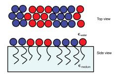
Figure 4.4. Cartoon of oppositely charged (red and blue denoting positive and negatively charged headgroups) molecules strongly absorbed to the interface. Molecules assume hexagonal close packing into periodic microphases as illustrated.
