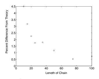
Figure 3.8. Percent difference in energy between theory and simulation at a reduced density  $\rho^* = 0.05$  and a reduced temperature  $T^* = 1.0$ . As the chain length is increased, percent difference decreases.
