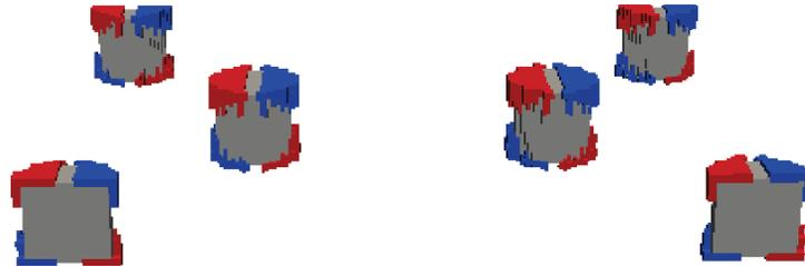
**Figure 4.9: Charge distributions at  $\Gamma_2$  resonance showing the charge accumulated at four corners of Al nanoparticles.**
