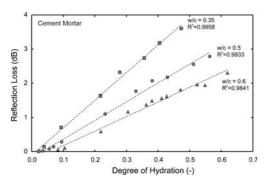
Fig. 10. Relationship between degree of hydration and reflection loss
