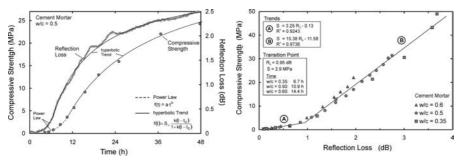
Fig. 5. Comparison of reflection loss and compressive strength of mortar with w/c = 0.5
