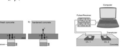
Fig. 1. Principle of HFWR-method
