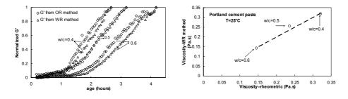
Fig. 8. Normalized dynamic storage shear moduli with WR and OR methods
