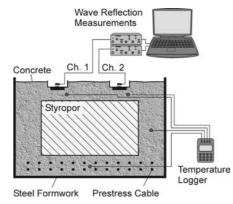
Fig. 12. Field measurements on box girder shortly after placing the concrete
