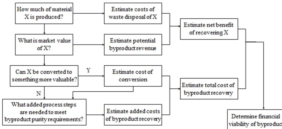
*Figure 2.* A simple flowsheet which describes the decision making process when determining potential uses of process byproducts. These byproducts may result in an expansion of the plant size, since additional processing may be economically beneficial for the company (Peters and Timmerhaus, 2003).
