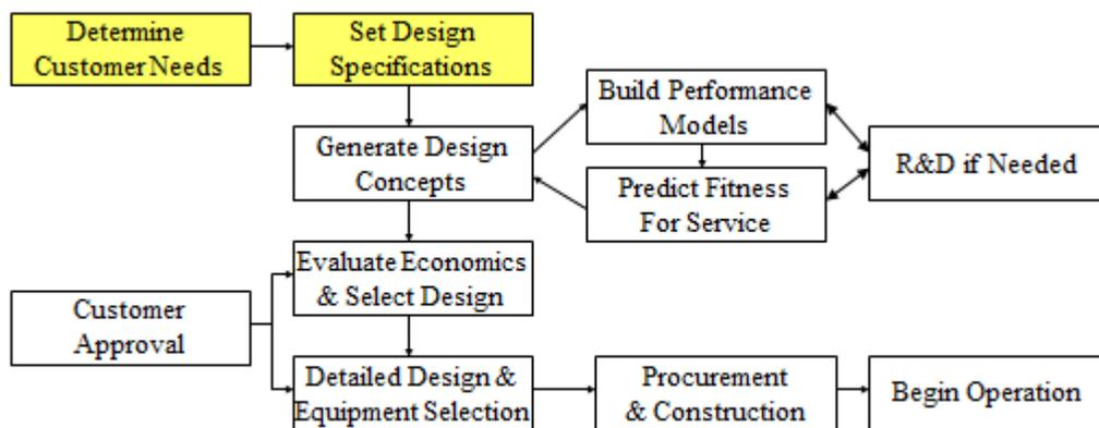
Figure 1. Early market analysis, shown here by the yellow boxes, will affect many elements of later design work, so it is important to produce a detailed report before taking further design steps (Towler and Sinnott, 2013).
