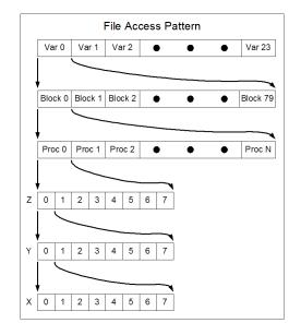
Figure 3.18. FLASH file datatype. This figure describes the hierarchy of the file datatype. At the highest level of the hierarchy, variables are contiguous. Within every variable, there are all the FLASH blocks from all the processors.
