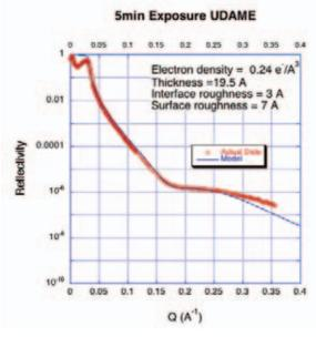
Figure 4: X-ray reflectivity spectra of five-minute exposed sample.
