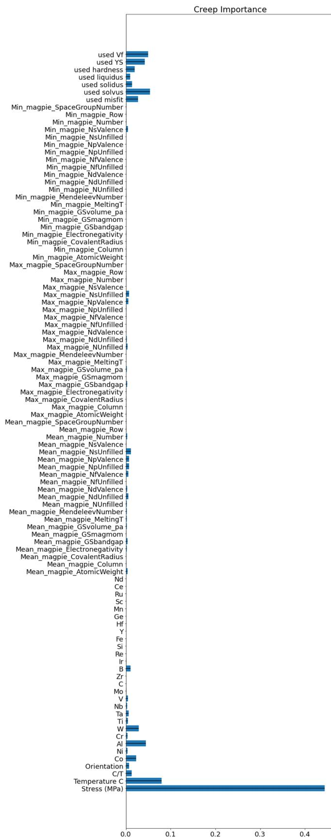
*Figure 6-21. Feature importance for predicting creep on the 16-alloy validation set.*
