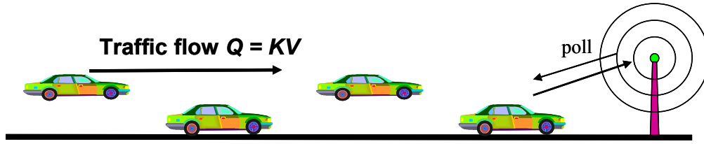
Figure 5.7: Bandwidth requirement of roadside sensor. With H = 10 hops, L = 4 lanes, P = 2000 bits, \tau = 2 seconds, the resulting bandwidth required is 40 Kbps.
