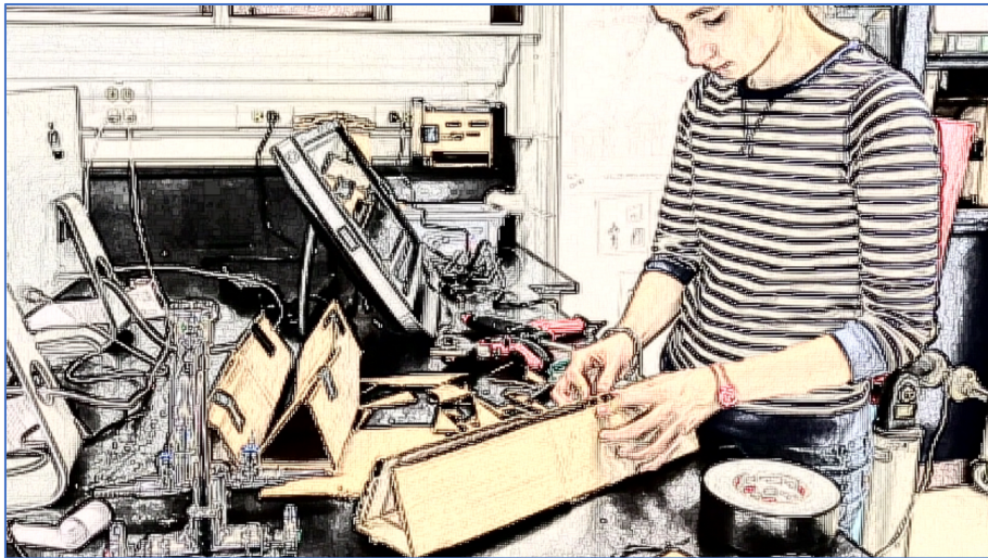
Figure 17. Using a cardboard cutter and duct tape to construct components of the chair.
