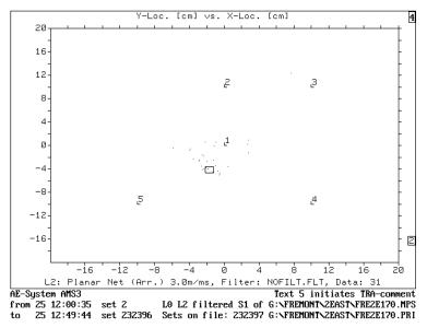
Figure 6 Source Location Plot for Site 2E 17 with Time Clustering
