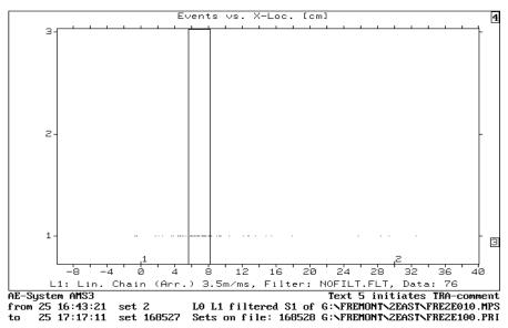
. Figure 13 Source Location Data for Test Site 10, Pier 2E
