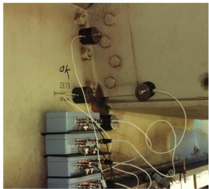
Figure 9 AE Setup on Pier 2W for Trapezoidal Attachments
