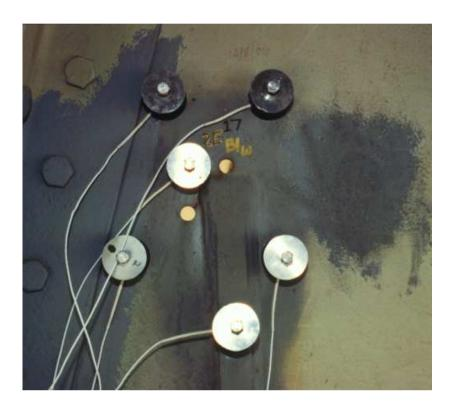
Figure 2 AE setup on test site 17 pier 2E
