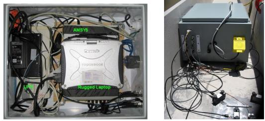
(a) Interior of enclosure showing AE unit, rugged laptop, and battery-backed power supply
