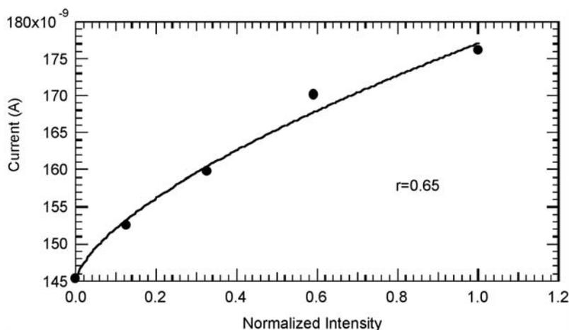
Figure 5: Current vs. intensity graph that measures the current response to varying light intensity.
