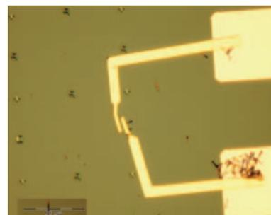
Figure 1: Gold electrode contacts made across a CdS nanowire through electron beam lithography.
