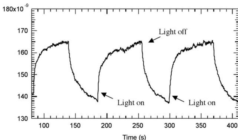
Figure 2: Current-over-time graph used to measure the photoresponse of the CdS nanowires to visible light.
