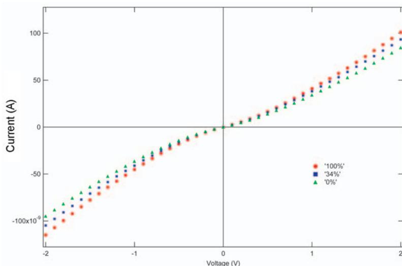
Figure 4: I-V graph that shows an increase in the current as the percentage of light intensity increases.
