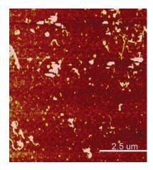
Figure 1. SEM image of SWNTs assembled on an MHA-coated nitride substrate.
