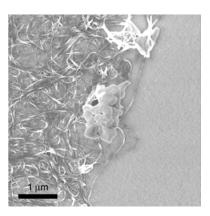
Figure 3. CNTs selectively assembled on MHA on a nitride substrate.
