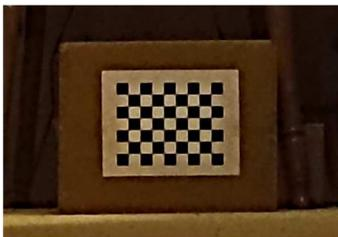
**Figure B-3: Chessboard target imaged by Phantom 3 for geometric calibration**
