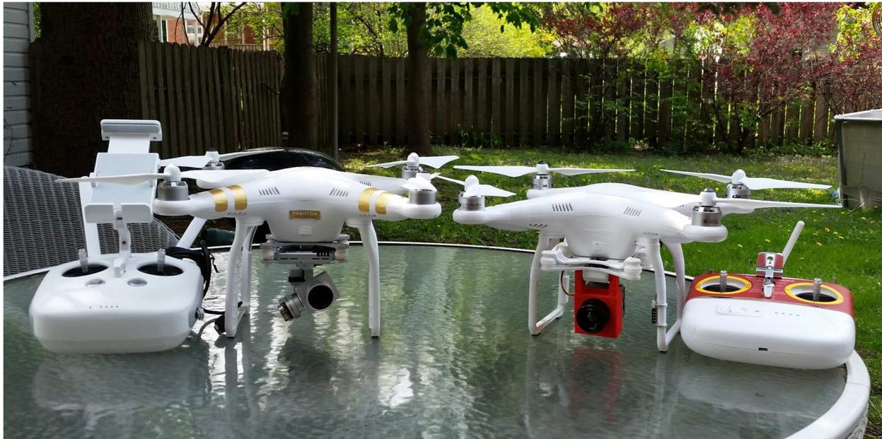
**Figure A-1: DJI Drones Used for Experiments. Phantom 3 with RGB Visible Band (left). Phantom 2 with LWIR Micro Bolometer (right)**
