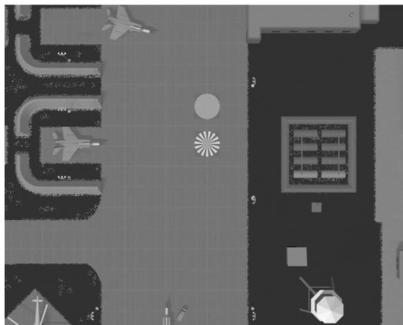
Figure 5-1a: Airport scene from DIRSIG rendered in the LWIR. LR image, with SNR = 40 dB, is up-sampled using BiCubic, IFEM, and VBI methods
