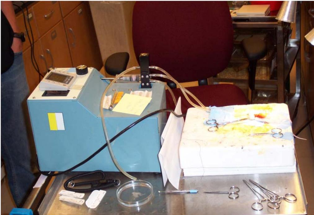
**Figure 28:** Ventilator used for intubating anesthetized mice.
