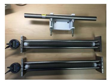
Figure 3.10 Set up of autogenous shrinkage test
