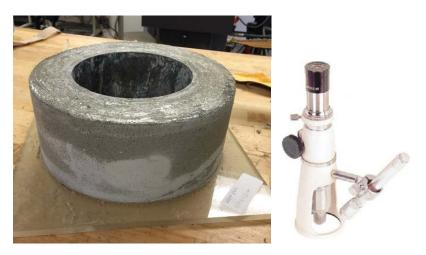
Figure 3.12 Restrained ring sample and portable microscope
