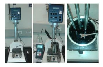
Figure 2.5 High-shear mixing of CNT and asphalt[16]
