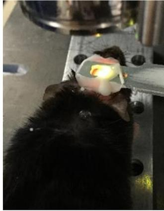
**Figure 5.2** A mouse is secured in the animal holder ready for vis-OCT imaging. The headbar is attached to the holder to reduce motion artifacts. The headbar has a center hole of  $5 \times 6 \text{ mm}^2$ .
