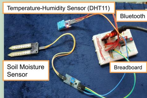
FIG. 3. CONNECTION BETWEEN BREADBOARD, BLUETOOTH, TEMPERATURE, HUMIDITY, AND SOIL MOISTURE SENSORS
