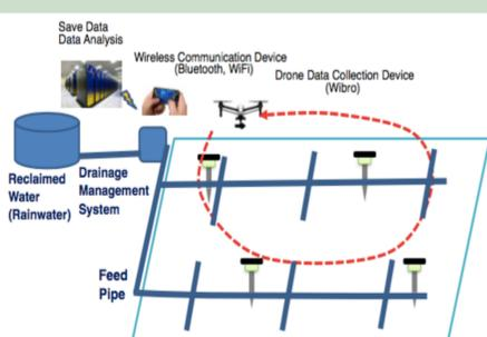
FIG. 2(B). MIMETIC DIAGRAM OF WATER MANAGEMENT USING RECLAIMED WATER
