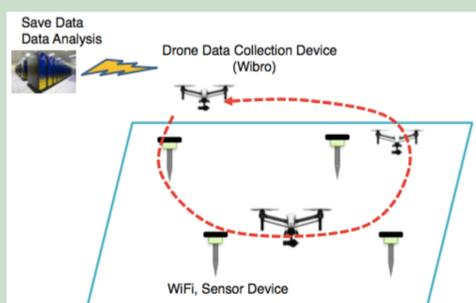
FIG. 2(A). MIMETIC DIAGRAM OF DRONE DATA COLLECTION
