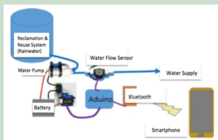
FIG. 15. CONNECTION THROUGHOUT WATER SUPPLY CONTROL
