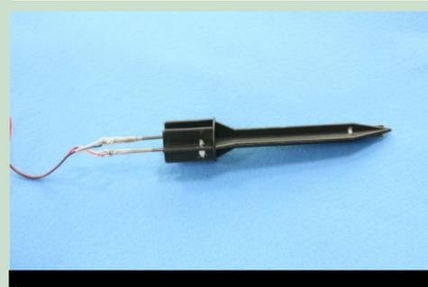
FIG. 5. ATTACHMENT OF SENSOR WIRES TO END OF CAST
