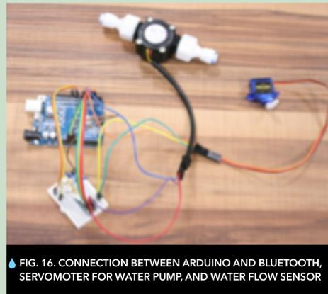
FIG. 16. CONNECTION BETWEEN ARDUINO AND BLUETOOTH, SERVO MOTOR FOR WATER PUMP, AND WATER FLOW SENSOR
