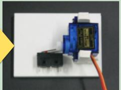
FIG. 18. DIAGRAM OF MICRO SWITCH WATER PUMP'S ON & OFF STATES → ACTIVATE MICRO SWITCH USING SERVO MOTOR
