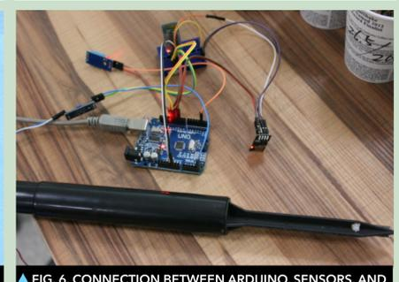
FIG. 6. CONNECTION BETWEEN ARDUINO, SENSORS, AND MODULE
