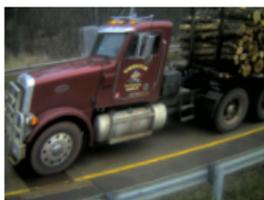
WIM Vehicle #9846 Class 12 **GVW 98.7 kip** length 57 ft 58 mph Lane 2 [\(expand\)](#)
