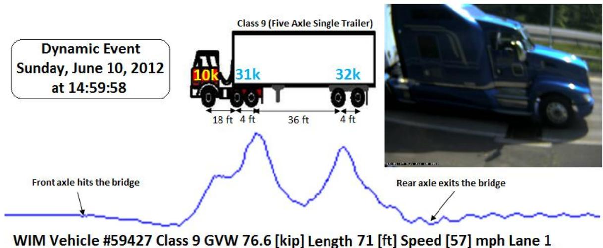
Figure 1.20: combined output of the WIM-SHM system.
