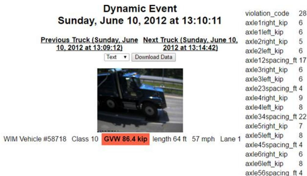
Figure 1.14: two types of WIM's output with axle configuration information.
