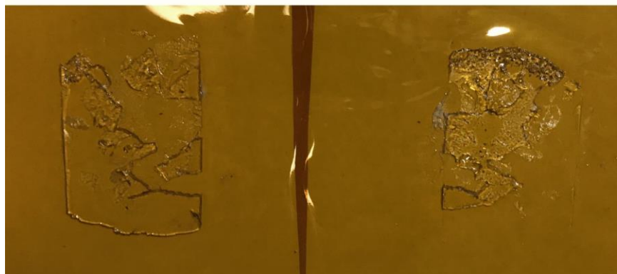
Figure 3-S6. Images of 1st molded Tetraol-20OH-Tin networks reprocessed under different conditions: (a) 140 °C, 70 min; (b) 120 °C, 15 min.
