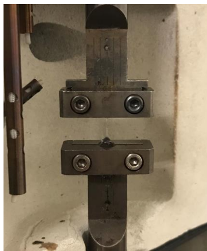
Figure 3-S5. Image of a PU sample after the high-temperature DMA test.
