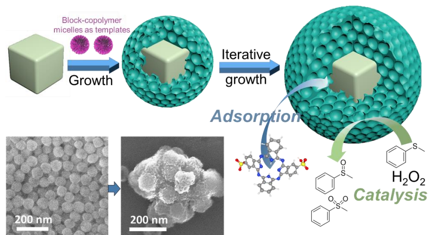
Figure 1.5 A HM-UiO-66 material synthetic strategy using UiO-66 nanoparticles as seeds and block copolymer micelles as templates, which resulted in materials with enhanced performances in adsorption and catalysis.
