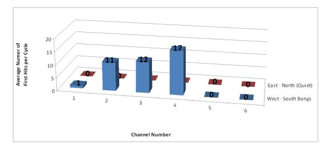
**Figure 5:** Comparison of first-hit results from high-energy AE events on the noisy west-south bascule girder and the quiet east-north bascule girder. Nearly all the high-energy AE events on the noisy bascule girder hit Channel 2, 3, or 4 first, indicating the events originated near the curved forging-bascule girder interface. No high-energy AE events were recorded on the quiet bascule girder.
