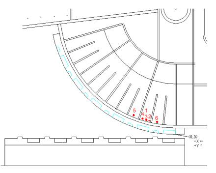
**Figure 10: AE array "D"** was deployed on the west leaf, south bascule girder for micro-localization of AE activity around the bolts connecting the curved upper forging to the bascule girder.
