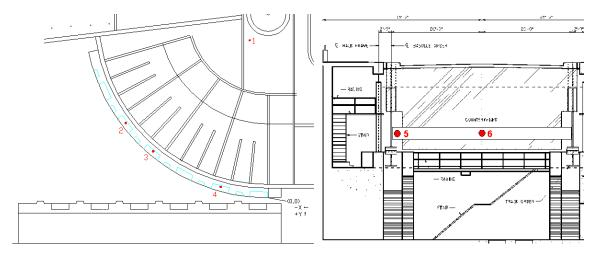
**Figure 6: AE array "B"** was deployed on the west leaf, with AE Sensors 1–4 on the south bascule girder and Sensors 5 and 6 on the transverse machinery strut. This array was used for comparison of AE activity from the north vs. south bascule girders.
