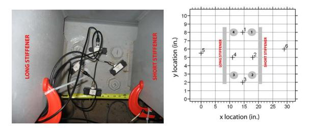
Figure 11: Photograph and drawing of array of AE transducers on bascule girder bolts near Location 4
