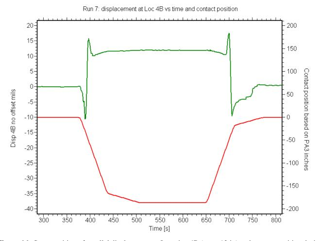
Figure 16: Superposition of parallel displacement at Location 4B (x = -12 in) and contact position during Run 7. Parallel displacement (green line) is given in mils. Contact position (red line, scale on right side of graph) is given in inches (arc length) along the rolling surface where x = 0represents the contact position when the leaf is fully closed. This repeatable, quasi-static behavior, is typical of all the test runs on the west leaf, south bascule girder.
