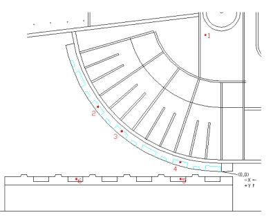
**Figure 3: AE array "A"** was deployed similarly on the west leaf, south bascule girder and east leaf, north bascule girder. This array was used for first-hit channel analysis.
