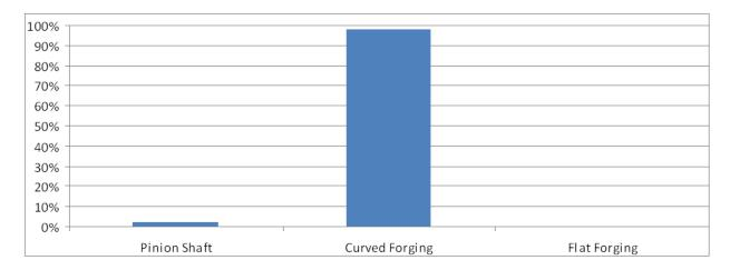
**Figure 4:** Results of first-hit analysis on the west leaf, south bascule girder. 98% of high-energy AE events hit Channels 2, 3, or 4 first, indicating that they originated near the curved forging-bascule girder interface. The balance originate near the pinion shaft; no high-energy AE events originate from the flat forging.
