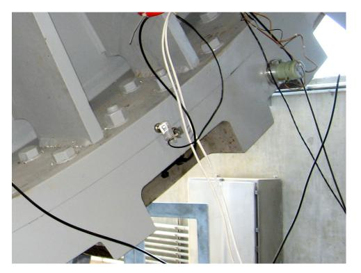
**Figure 13:** Eddy-current displacement sensor pair (metal bracket with inverted B on label) deployed across bascule girder-curved forging interface. The electronic clinometer (tiltmeter), a greyish cylinder magnetically mounted to the curved bottom forging, is also visible. All instrument cables were tied off to clamps on the bascule girder for strain relief.
