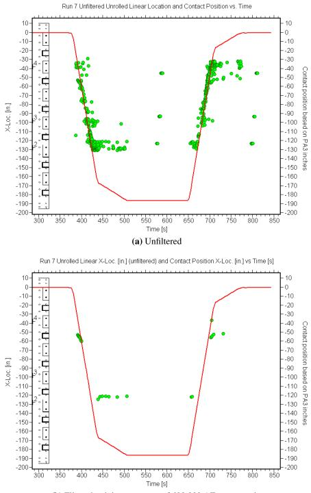
(b) Filtered, minimum energy of 600,000 AE energy units
