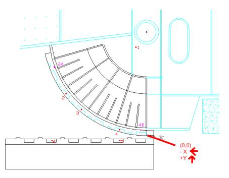
Figure 1: Overview of bascule girder/track area showing primary (Array A) sensor locations and the coordinate system used in analysis. Note that for planar location along the bascule girder, the coordinate system rotates and translates with the movement of the bridge; i.e., the coordinate system is defined by sensors 2, 3, and 4. Locations 2A and 4B were used exclusively for the displacement measurements described in Analysis #5.
