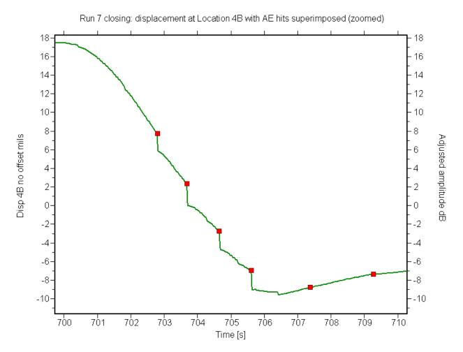
**Figure 18:** Close-up of Run 7 closing parallel displacement at Location 4B with AE events with energy greater than 600,000 AE energy units superimposed. As with Figure 17, the AE amplitudes have been arbitrarily offset and are meaningless. Note that each "jump" in the displacement data is accompanied by a high-energy AE event; this is typical of most of the events shown in Figure 17.
