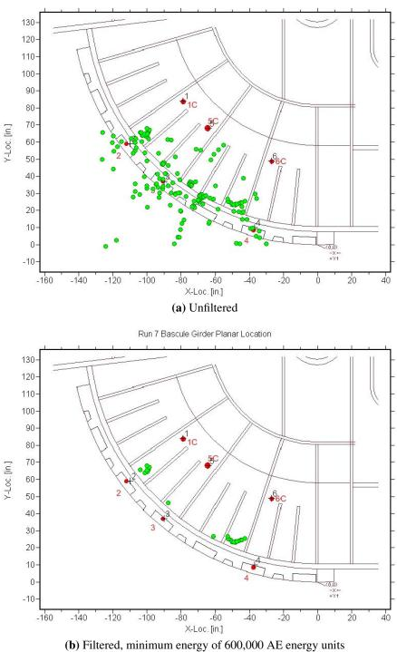
**Figure 9:** Planar location along the upper forging during opening and closing of the west leaf in Run 7, unfiltered (a) and filtered (b).
