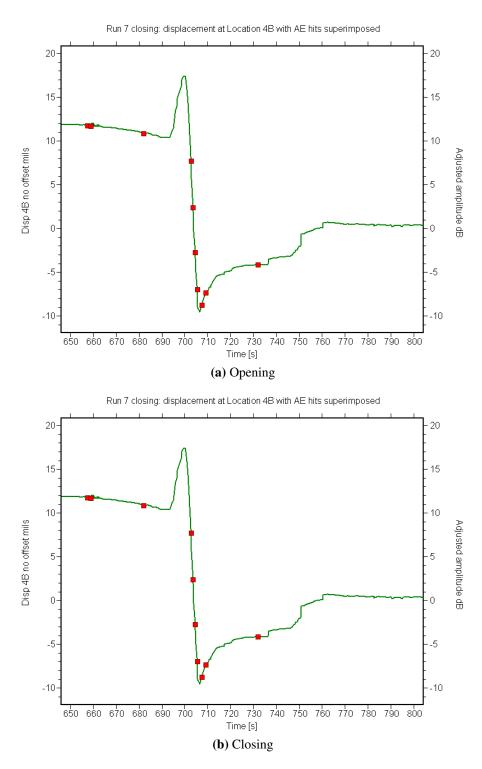
**Figure 17:** Run 7 parallel displacement at Location 4B with AE events with energy greater than 600,000 AE energy units superimposed. AE amplitudes have been arbitrarily offset to generally follow the displacement plot for comparison purposes; the amplitudes displayed are meaningless.
