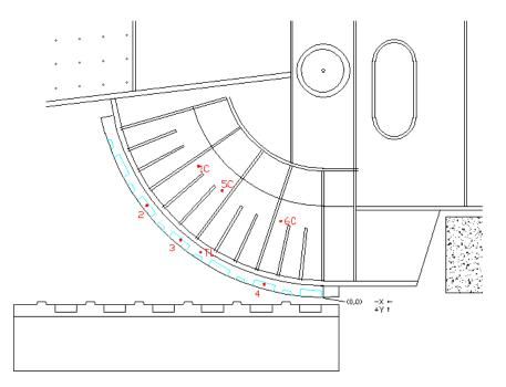
**Figure 7: AE array "C"** was deployed on the west leaf, south bascule girder for linear location analysis by "unrolling" the curved upper forging on the bascule girder. The three sensors closest to the pinion were used as guard sensors to intercept noise not coming from the curved forging.
