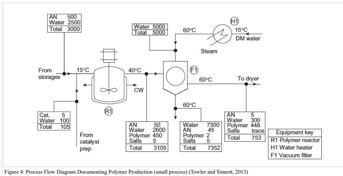
Figure 4: Process Flow Diagram Documenting Polymer Production (small process) (Towler and Sinnott, 2013)
