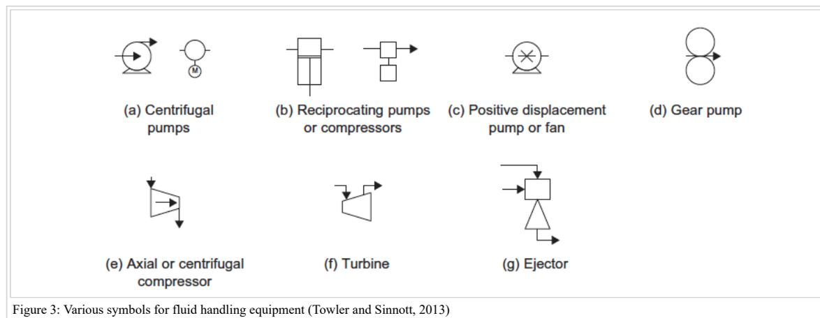
Figure 3: Various symbols for fluid handling equipment (Towler and Sinnott, 2013)
