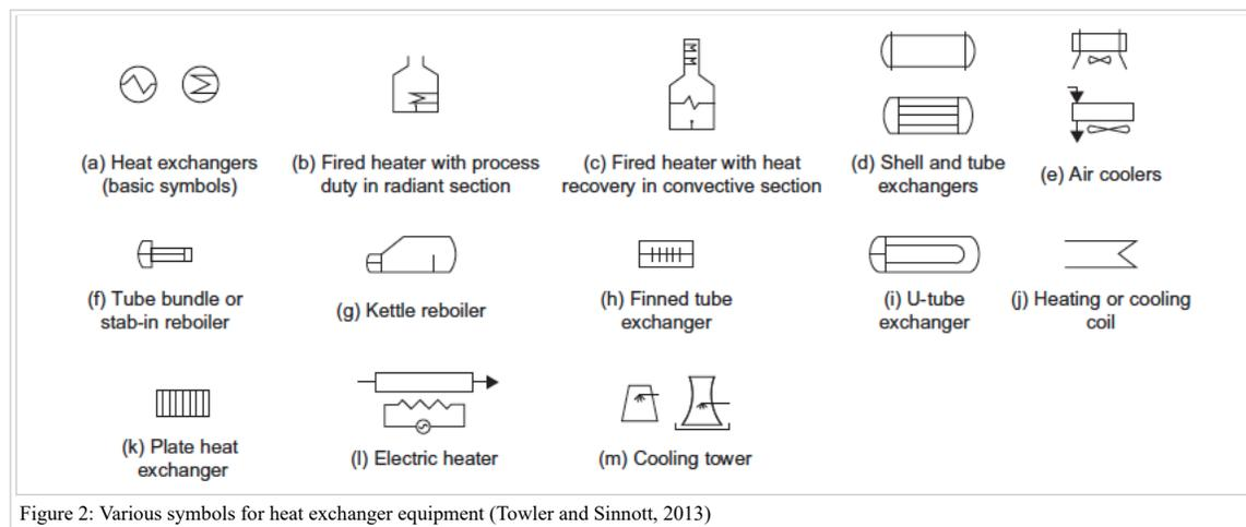
Figure 2: Various symbols for heat exchanger equipment (Towler and Sinnott, 2013)
