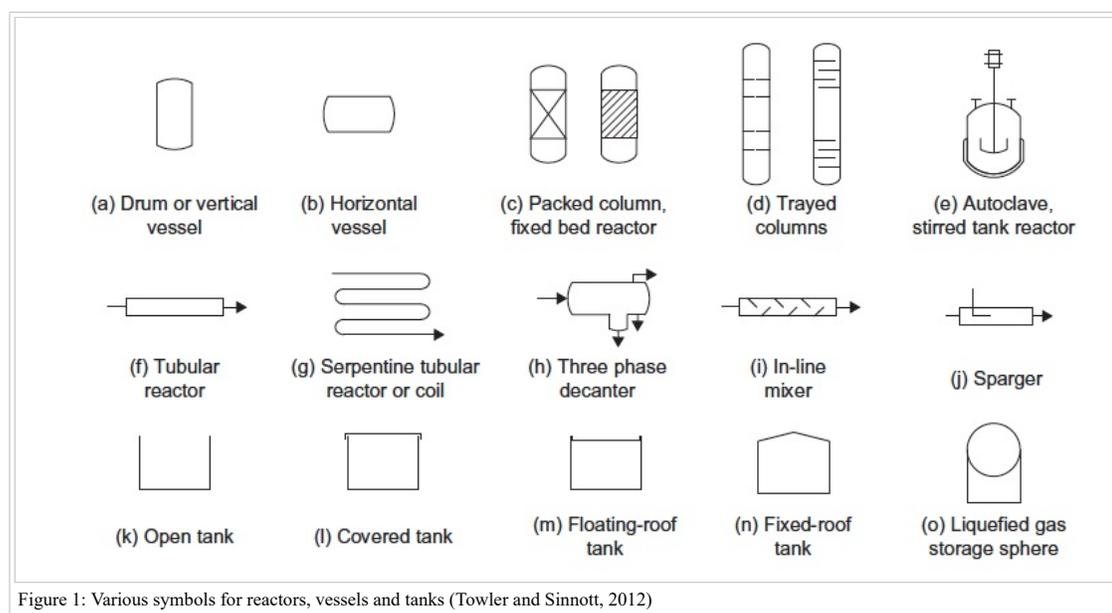
Figure 1: Various symbols for reactors, vessels and tanks (Towler and Sinnott, 2012)
