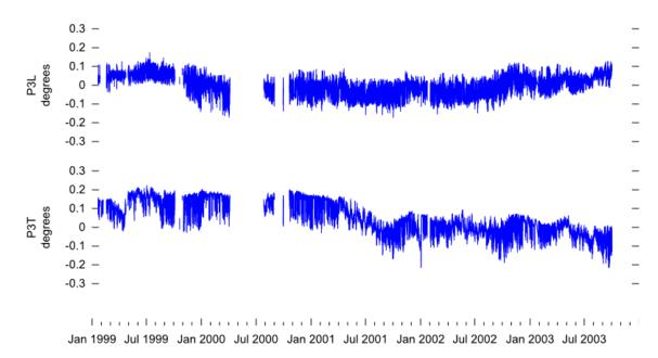
Figure 4: Time history of typical longitudinal and transverse response of a pier
