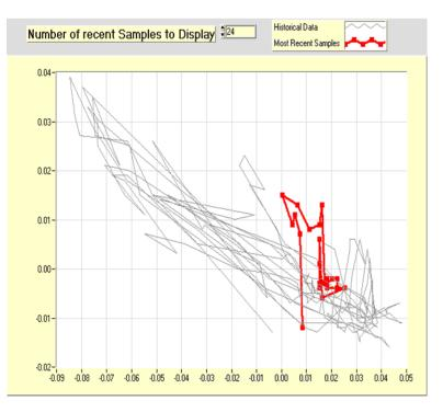
**Figure 5:** Typical longitudinal response plotted against transverse response. The most recent data are highlighted for easy comparison to the historical record.
