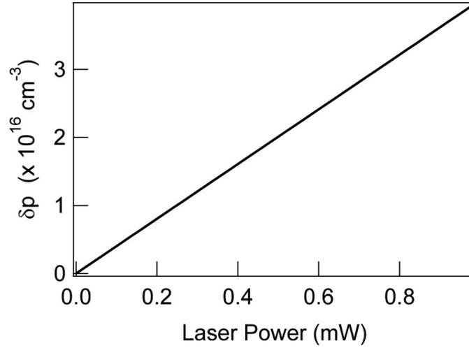
Figure 5.1. Excess hole concentration versus laser power for a 50 nm silicon nanowire.
