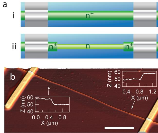
Figure 5.6. Surface etching of n-Si nanowire devices. (a) Top-down schematic of an etched device before, (i), and after, (ii), surface etching. (b) AFM image of a device after surface etching. Line profiles show the change in height at each side of the etched region. The scale bar is  $3 \mu m$ .
