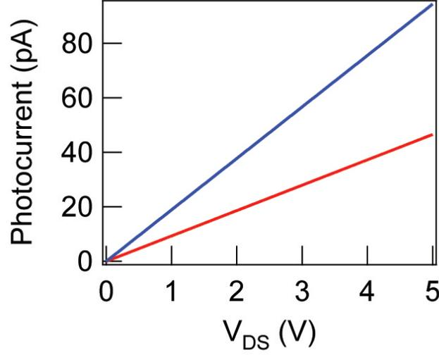
Figure 5.4. Calculated photocurrent versus applied bias for uniform silicon nanowire devices. Parameters for the calculations for each curve are as follows. Red:  $R=550\text{ k}\Omega$ ,  $L=13\text{ }\mu\text{m}$ ,  $w=500\text{ nm}$ ,  $A=7.85\times 10^{-11}\text{ cm}^2$ , and  $\mu_h = 100\text{cm}^2/\text{Vs}$ . Blue:  $R=2\text{ M}\Omega$ ,  $L=10\text{ }\mu\text{m}$ ,  $w=500\text{ nm}$ ,  $A=7.85\times 10^{-11}\text{ cm}^2$ , and  $\mu_h = 120\text{cm}^2/\text{Vs}$
