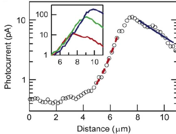
Figure 2.14. SPCM line profiles of a CdS device. Main image is a semi-logarithmic plot of the photocurrent profile taken at 1 V applied bias. The dashed and solid lines are exponential fits to the data. The inset shows line profiles taken at different biases. The slope of the signal decay does not change significantly between scans. Taken from Gu et al.<sup>68</sup>
