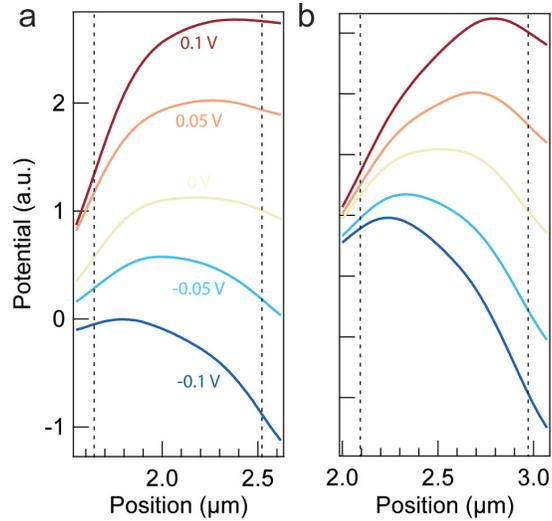
Figure 7.5. Pseudo potential profiles taken from SPCM data of p-type nanowire FETs at the tip, (a), and base, (b), of a boron-doped silicon nanowire. Dashed lines indicate the position of the intruded metal-semiconductor junctions. Voltage values in ‘a’ are the applied source-drain bias.
