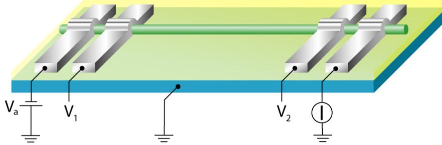
Figure 3.4. Schematic of a four-probe nanowire device.
