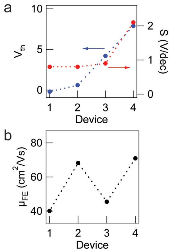
Figure 7.2. Device parameters for p-type silicon nanowire FETs along the nanowire length. (a) Threshold voltage,  $V_{th}$ , (left axis) and subthreshold slope,  $S$ , (right axis) for devices 1 to 4. (b) Field-effect mobility for devices 1 to 4. The nanowire tip is closest to device 1 with 4 being near the base of the nanowire.
