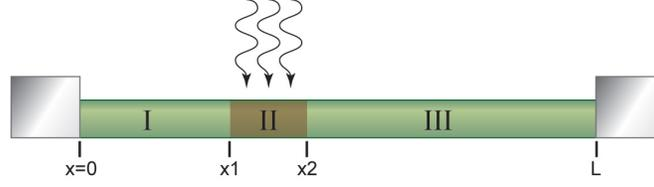
Figure 5.2. Diagram of a nanowire device showing regions used for excess carrier distribution calculations.
