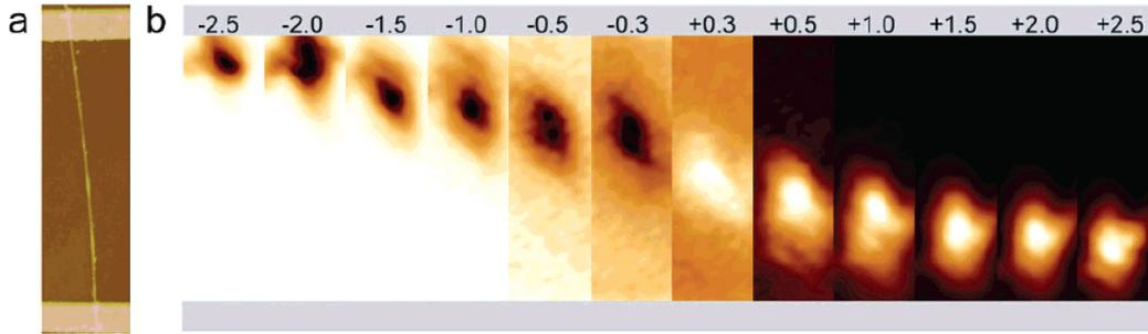
Figure 2.13. SPCM imaging of a CdS nanowire device with two ohmic contacts. (a) AFM topographic image of the CdS nanowire device. Device channel length is  $11 \mu m$  (b) Sequence of SPCM images with the top electrode biased as indicated. Taken from Gu et al.<sup>68</sup>
