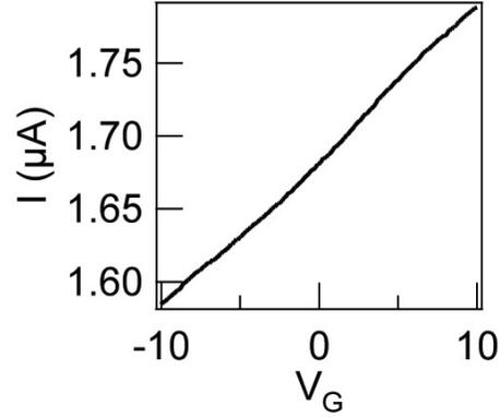
Figure 3.6. Transfer curve for a heavily doped n-Si nanowire device. The field-effect mobility estimated from this device is  $38 \text{ cm}^2/\text{V}\cdot\text{s}$ .
