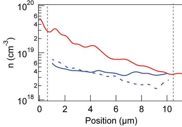
Figure 5.11. Effective electron concentration profiles calculated from the quantitative potential profiles in Figure 5.10a (red) and Figure 5.10b (blue). Solid profiles are averaged over the applied bias range of -4 V to 1 V. The dashed profile is taken from the potential profile of the etched device at 5 V.
