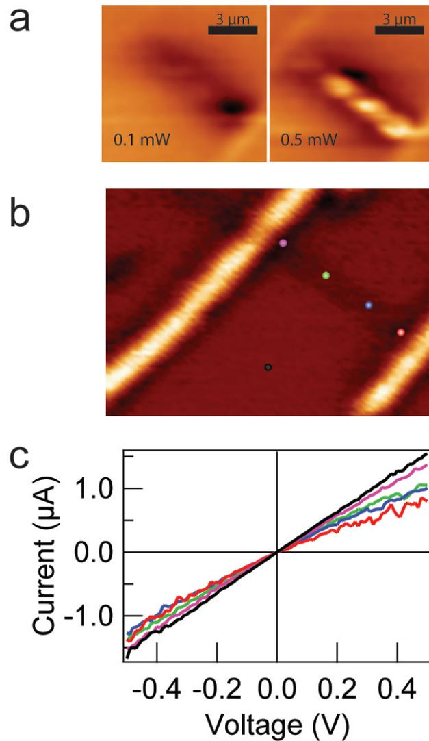
Figure B.2. Negative photoconductivity in InAs nanowire devices. (a) SPCM images of an InAs nanowire device with 10 mV applied bias taken at 0.1 mW (left) and 0.5 mW (right). (b) Reflection image with colored dots marking the location of excitation for the I-V data presented in 'c'. (c) I-V data taken under local illumination. The color of each curve corresponds to the dots in 'b' that indicate the location of the laser spot.
