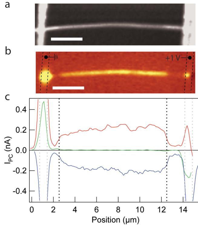
Figure 5.8. SPCM analysis of an n-Si nanowire device with etched channel. (a) Reflection image of the nanowire device and corresponding SPCM image, (b), taken with 1 V bias applied to the right contact. (c) Line profiles taken along the device channel for SPCM scans at 1 V (red), 0 V (green), and -1 V (blue). Vertical dashed black lines mark the extent of the etched region and the location of the metal contacts are indicated by the dashed gray lines. Scale bars are 3  $\mu\text{m}$ .
