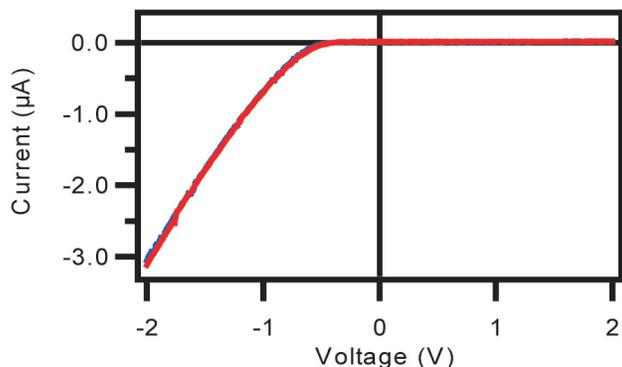
Figure 4.9. Current vs. voltage data from an n-type silicon nanowire Schottky diode before (red) and after (blue) EBIC analysis
