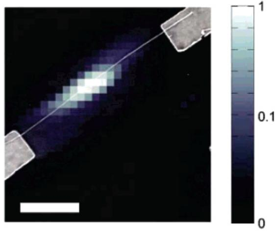
Figure 2.10. Normalized photocurrent map of a p-i-n silicon nanowire avalanche photodiode. Bright contrast corresponds to an increase in device current. Bias voltage was -28 V. Scale bar is  $2 \mu m$ . Taken from Yang et al.<sup>10</sup>
