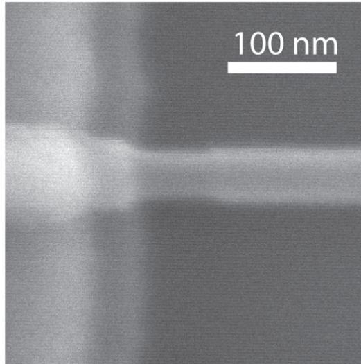
Figure 4.7. SEM image of the near-contact region of a nanowire device fabricated with an oxidized silicon nanowire.
