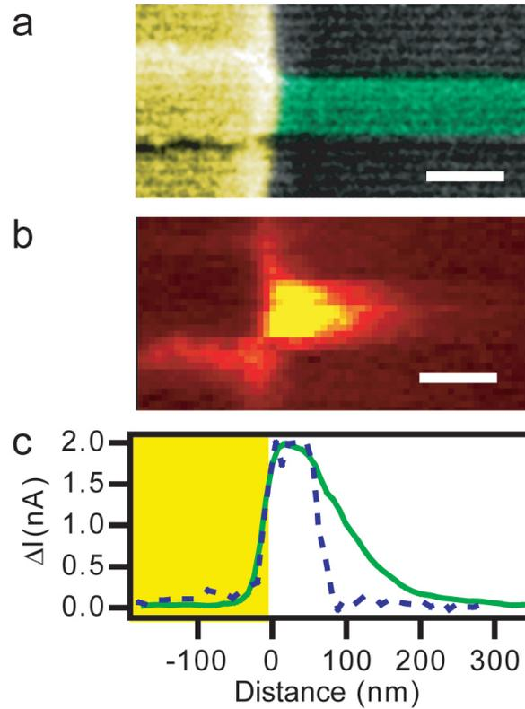
Figure 4.3. EBIC measurement of a nanowire Schottky diode. (a) False-color SEM image of the nanowire device near the Schottky contact. (b) EBIC signal from the region in ‘a’. Bright contrast indicates an increase in current. (c) Line profiles of the EBIC data in ‘b’ taken along the nanowire axis (solid line) and across the nanowire (dashed line). Scale bars are 100 nm.
