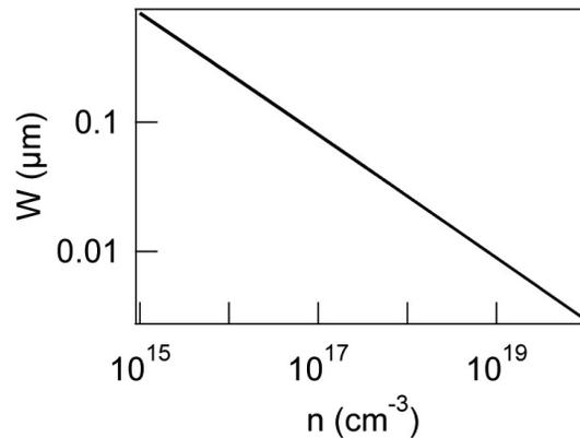
Figure 7.4. Depletion width versus electron concentration for an unbiased p-Si - NiSi Schottky barrier.
