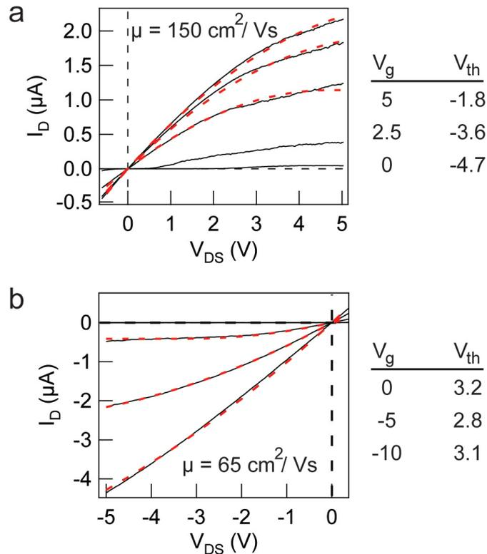
Figure 6.2. I-V data for etched n-Si, (a), and unetched p-Si, (b), nanowire FETs at different gate biases. Red dashed lines are fits to the data using the quadratic model for MOSFET drain current. The table to the right of each plot gives the applied gate bias and the threshold voltage determined from the fits.
