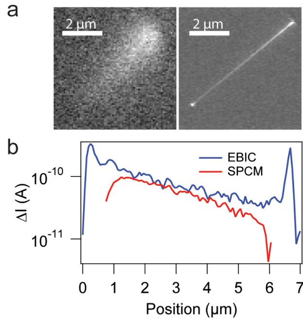
Figure A.1. Comparison of EBIC and SPCM measurement of an n-Si ohmic nanowire device. (a) EBIC and SPCM image of the same nanowire device. Scans were taken at 0.5 V applied bias. (b) Line profiles of the data in 'a' taken along the nanowire axis.
