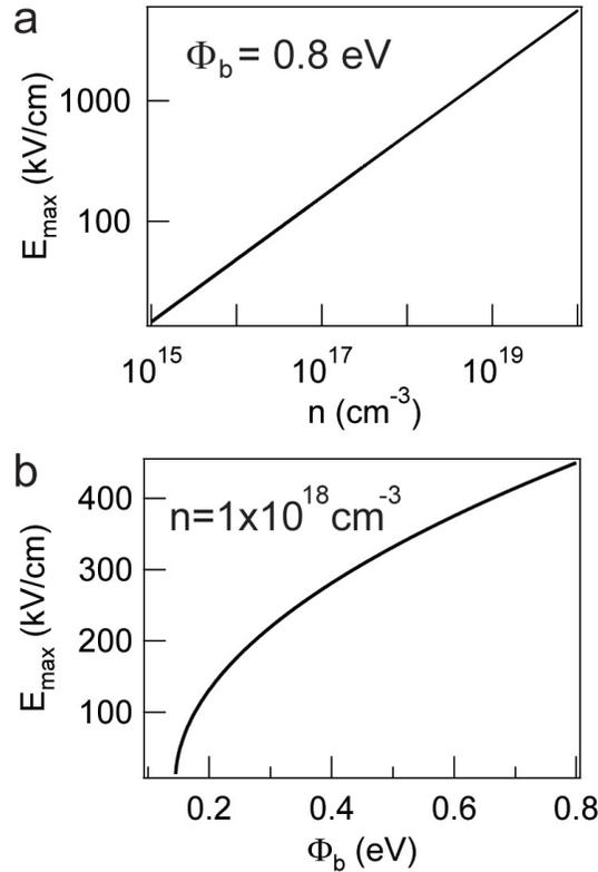
Figure 8.2. Maximum electric field at the Au-Si interface for an ideal Schottky barrier. (a)  $E_{\max}$  versus electron concentration for the ideal Au-Si barrier height of 0.8 eV. (b)  $E_{\max}$  versus Schottky barrier height at  $n = 1 \times 10^{18} \text{ cm}^{-3}$ .
