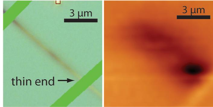
Figure B.1. SPCM measurements of an InAs nanowire device showing the effect of taper. Optical image of the device, (a), and corresponding local photocurrent map, (b). Applied bias was -10 mV. Dark contrast represents a positive photocurrent response. Significantly enhanced signal is observed at the thin end of the nanowire device.
