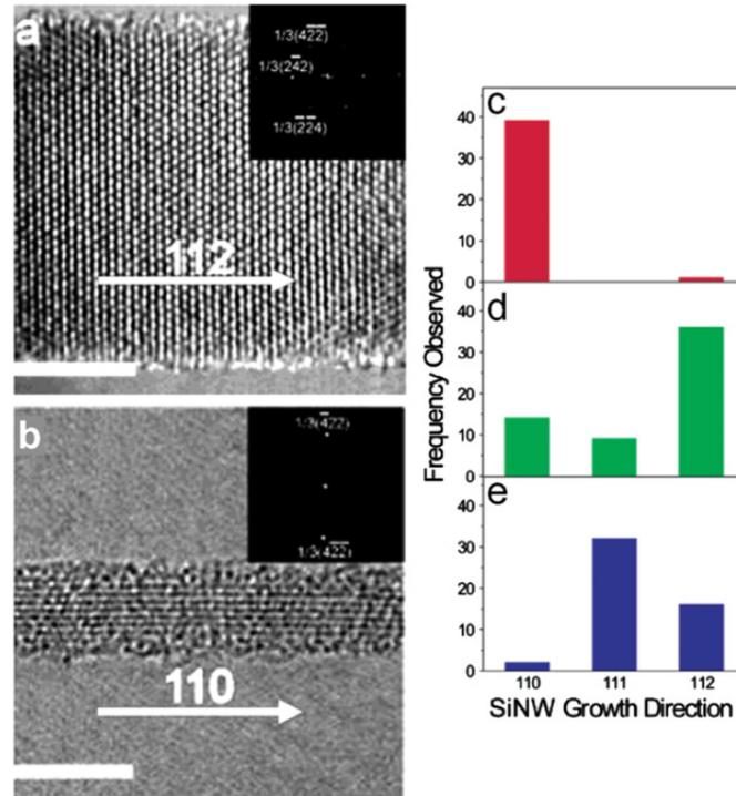
Figure 2.1. Silicon nanowire crystallinity and growth direction. (a) and (b) HRTEM images of silicon nanowire with diameters of 12.3 nm and 3.5 nm respectively. Wires are single crystal. Scale bars are 5 nm. (c)-(e) Histogram of the growth directions for silicon nanowires with diameters from 3 to 10 nm (c), from 10 to 20 nm (d) and from 20 to 30 nm (e). Taken from Lu and Lieber<sup>5</sup>.
