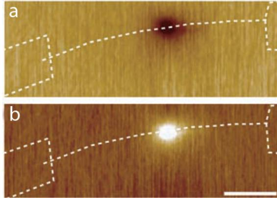
Figure 2.9. SGM images of an  $n^+ - n - n^+$  modulation-doped nanowire. (a) and (b) were recorded with a tip bias of  $-9\text{ V}$  and  $+9\text{ V}$ , respectively. Source-drain bias was  $1\text{ V}$ . The dark and bright regions correspond to reduced and enhanced conductance, respectively. The white dashed lines highlight the positions of the nanowire and electrodes. Scale bar is  $1\ \mu\text{m}$ . Taken from Yang et al.<sup>31</sup>
