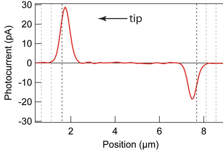
Figure 7.6. SPCM line profile of an unbiased long-channel silicon nanowire p-FET. Grey dashed lines mark the position of the lithographically defined contacts while black dashed lines mark the metal-semiconductor junction of the intruded contacts.
