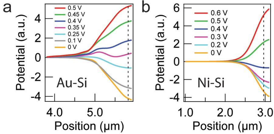
Figure 8.5. SPCM determination of  $V_{bi}$  in nanowire Schottky diodes. (a) Pseudo potential profiles of a Au-Si nanowire Schottky diode at the indicated forward biases ( $V_{bi} \approx 0.35$  V). (b) Pseudo potential profiles of a Ni-Si nanowire Schottky diode at the indicated forward biases ( $0.4$  V  $< V_{bi} < 0.5$  V).
