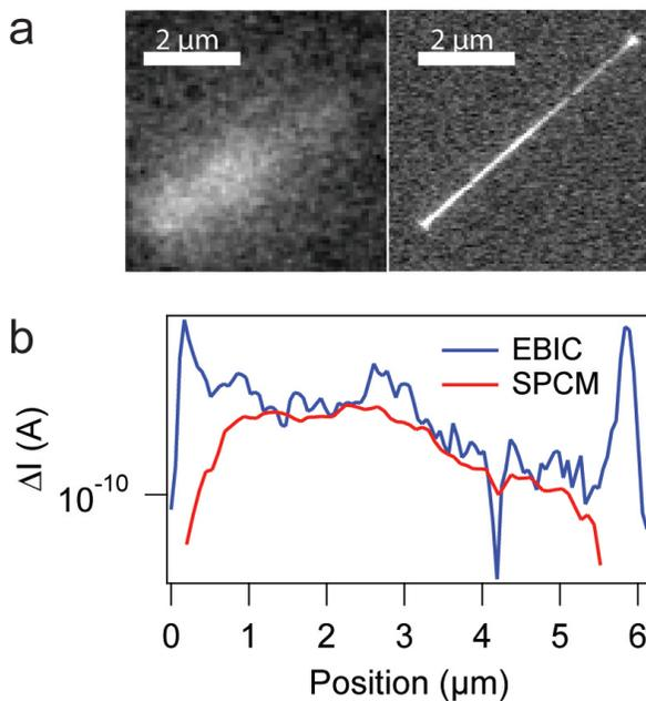
Figure A.2. Comparison of EBIC and SPCM measurement of an n-Si ohmic nanowire device. (a) EBIC and SPCM image of the same nanowire device. Scans were taken at 1 V applied bias. (b) Line profiles of the data in 'a' taken along the nanowire axis.
