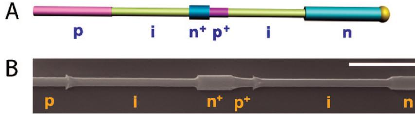
Figure 2.2. Axial modulation doping in a silicon nanowire. (a) Schematic of a functional modulation-doped nanowire structure consisting of two p-i-n diodes in series. (b) SEM image after selective etching of an axially modulated p-i-n<sup>+</sup>-p<sup>+</sup>-i-n silicon nanowire. Scale bar is 1  $\mu\text{m}$ . Taken from Kempa et al.<sup>36</sup>
