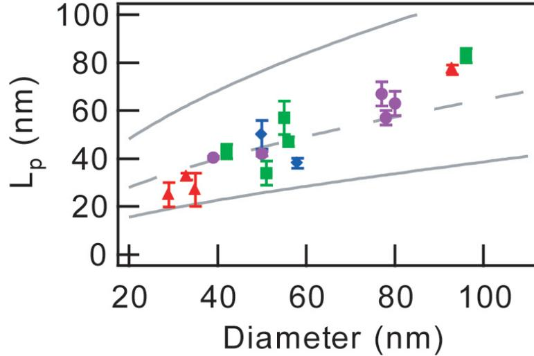
Figure 4.5. Plot of  $L_p$  versus diameter for varying gas-phase Si:P doping ratios: 500:1 (red triangles), 1000:1 (green squares), 1500:1 (blue diamonds), 2000:1 (magenta circles). Grey lines are model calculations of  $L_p$  vs diameter for various values of the surface recombination velocity,  $S$ . Top, bottom and dashed lines correspond to  $S = 1 \times 10^5 \text{ cm s}^{-1}$ ,  $1 \times 10^6 \text{ cm s}^{-1}$  and  $3 \times 10^5 \text{ cm s}^{-1}$ , respectively.
