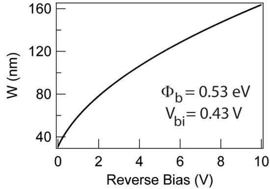
Figure 8.6. Depletion width of a Ni-Si Schottky barrier versus applied reverse bias. Parameters for the calculation were taken from the estimates in the main text.
