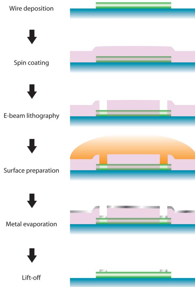
Figure 3.2. Nanowire device fabrication process flow.
