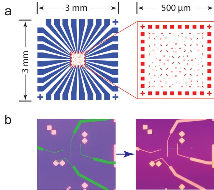
Figure 3.1. Nanowire device alignment and contact design. (a) Photolithography pattern and dimensions for a typical device substrate. (b) First image shows the location of two nanowires and contacts designed in CAD software. Second image shows the completed devices after EBL.
