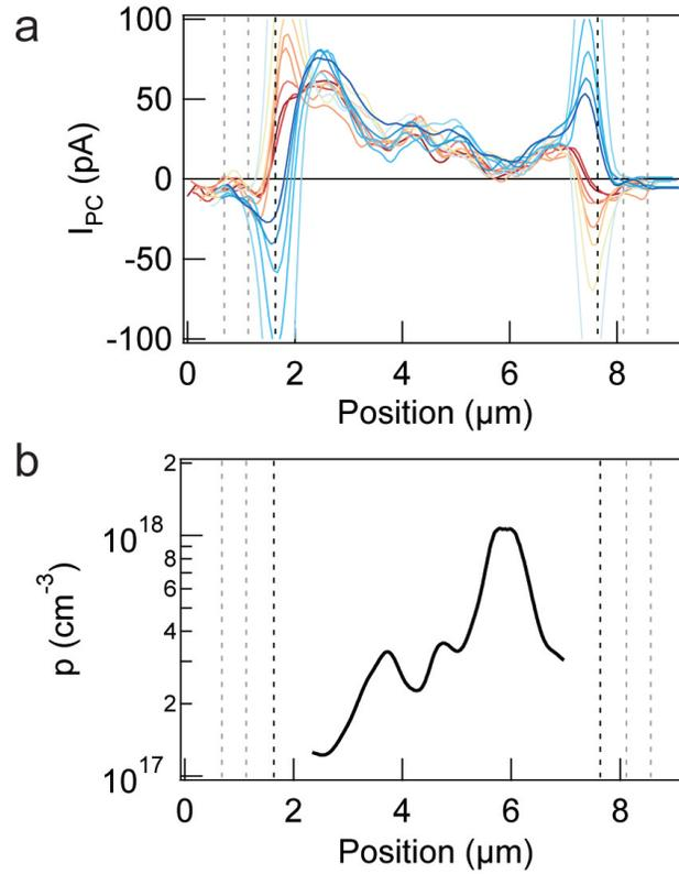
Figure 7.8. SPCM line profiles at low to moderate source-drain bias and extracted effective hold concentration. (a) Bias-normalized SPCM line profiles taken from  $-0.5 V_{DS}$  to  $0.8 V_{DS}$  in increments of  $0.1 V$ . Grey dashed lines mark the position of the lithographically defined contacts while black dashed lines mark the metal-semiconductor junction of the intruded contacts. (b) Extracted effective hole concentration within the device channel.
