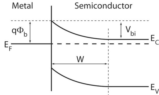
Figure 8.1. Band structure diagram of a Schottky barrier to an n-type semiconductor.
