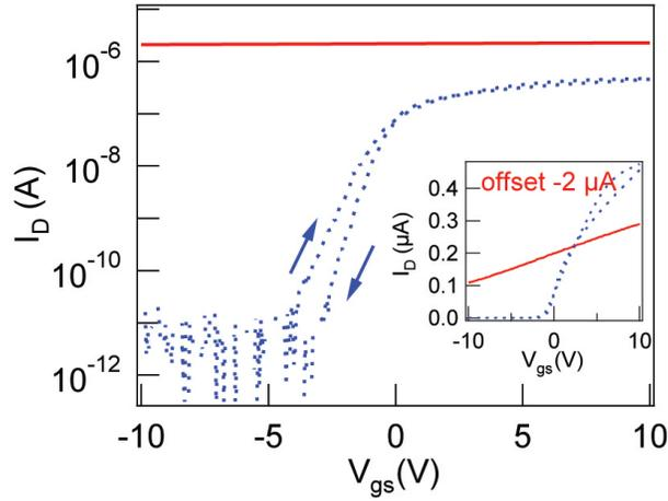
Figure 6.1. Device transfer curves of an n-Si nanowire FET before (red, solid) and after (blue, dashed) etching. The main plot is on a semi-log scale to show the subthreshold characteristics while the inset is on a linear scale to demonstrate the improvement in conductance. The before etching data is offset by  $-2 \mu\text{A}$  on the linear scale for comparison. Arrows on the main plot indicate sweep direction.
