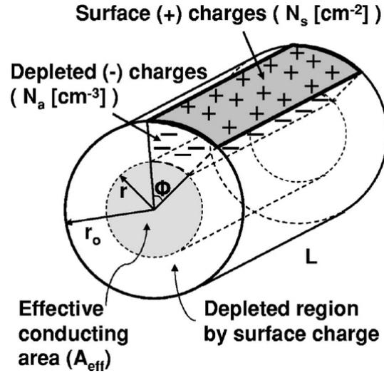
Figure 2.8. Schematic showing depletion near the nanowire surface caused by surface charge. Taken from Seo et al.<sup>49</sup>
