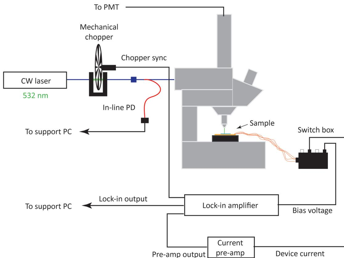
Figure 3.7. Schematic of the experimental setup for SPCM measurements.
