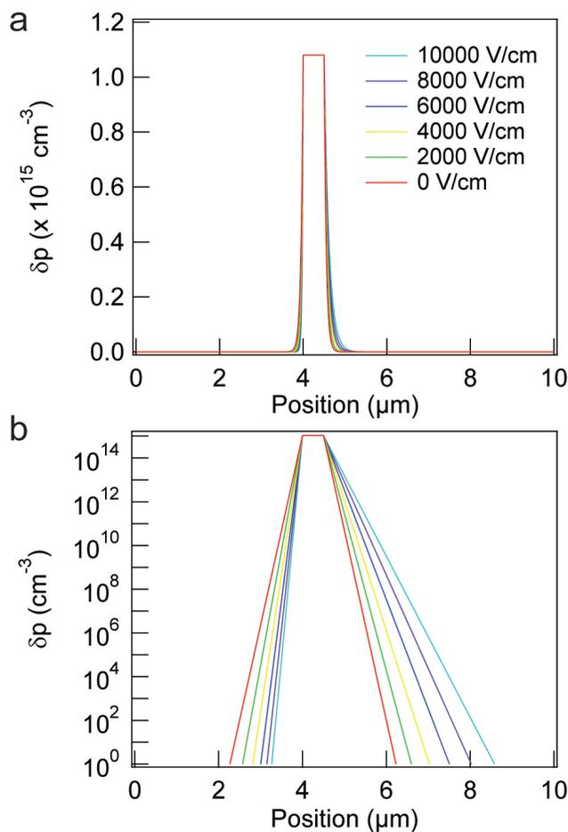
Figure 5.3. Calculated excess hole distributions for electric fields from 0 V/cm to 10,000 V/cm. Data is plotted on a linear scale, (a), and a semilogarithmic scale, (b).
