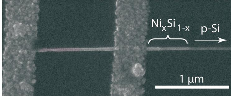
Figure 3.3. SEM image of an intruded silicide contact in a p-Si nanowire.
