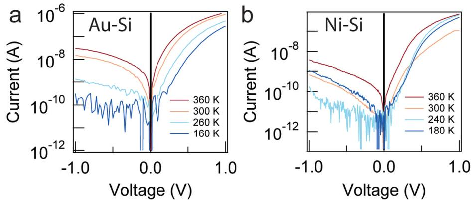
Figure 8.4. Current versus applied voltage at various temperatures for Au-Si, (a), and Ni-Si, (b), Schottky diodes.
