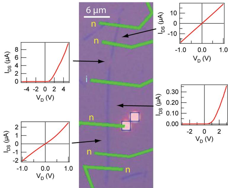
Figure 8.3. Schottky diodes fabricated from modulation-doped silicon nanowires. Devices fabricated at either end of the nanowire show symmetric I-V behavior while those with a contact on the middle segment show rectifying behavior.
