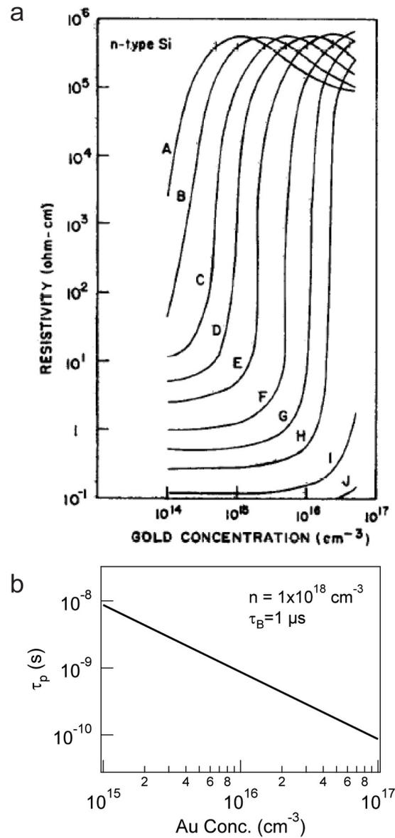
Figure 2.4. Effects of Au contamination in Si. (a) Calculated resistivity vs. gold concentration for n-type silicon at 300 K. A-J are calculated with increasing phosphorus concentrations ( $\text{cm}^{-3}$ ) from  $1 \times 10^{14} \text{ cm}^{-3}$  to  $1 \times 10^{17} \text{ cm}^{-3}$ . Taken from Bullis<sup>43</sup>. (b) Calculated minority carrier lifetime vs. gold concentration for n-type silicon at 300 K. Expression for the calculation was taken from Fairfield and Gokhale<sup>44</sup>.
