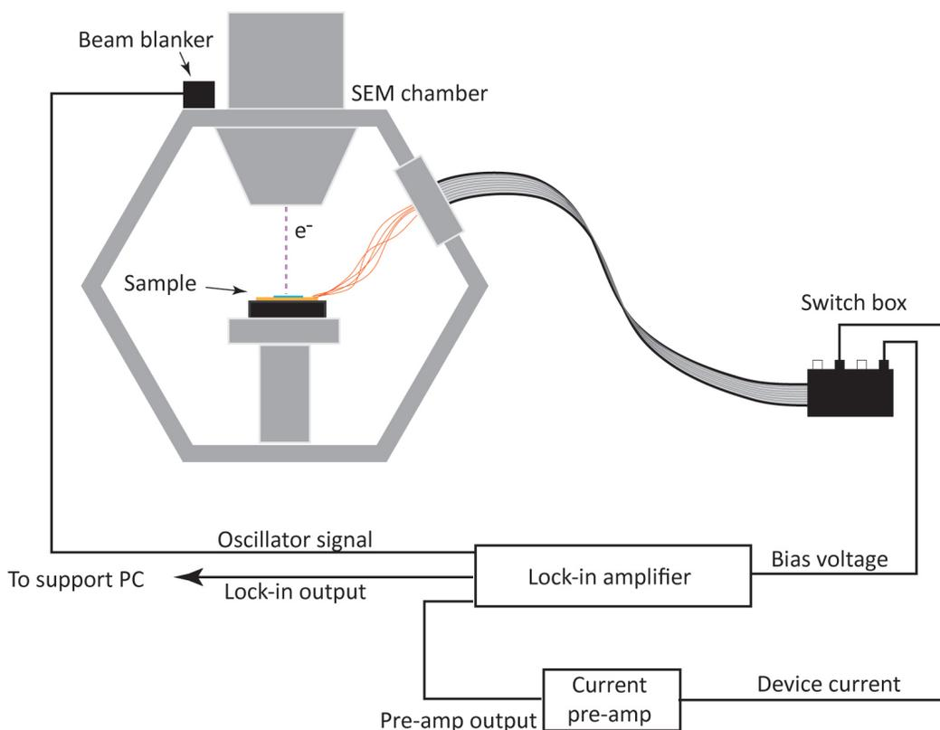
Figure 3.8. Schematic of the experimental setup for EBIC measurements.
