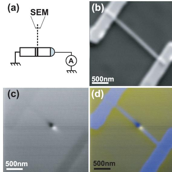
Figure 2.11. Location of nanowire heterojunctions using EBIC. (a) Schematic of the EBIC measurement. (b) SEM image of an InAs nanowire device with two 12 nm InP barriers separated by a 12 nm InAs region in the center of the channel. (c) EBIC map of the device in 'b'. (d) Composite image of 'b' and 'c' showing the location of the EBIC signal. Between the bright and dark contrast is the location of the InAs quantum dot. Taken from Gustafsson et al.<sup>62</sup>
