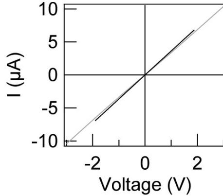
Figure 3.5. Four-probe (black) and two-terminal (red) I-V data for an n-Si nanowire device. From this plot the total series resistance introduced by the contacts is  $16 \text{ k}\Omega$ .
