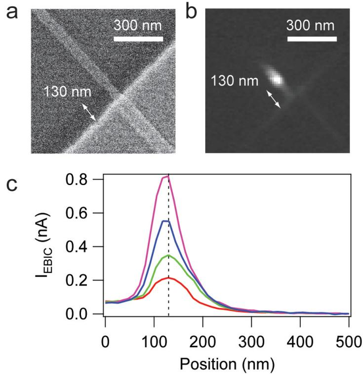
Figure 4.12. Effect of the MMA undercut on EBIC analysis of silicon nanowire Schottky diodes. (a) SEM image showing the extent of the undercut and, (b), the corresponding EBIC image taken at 2 V reverse bias. (c) Line profiles of the EBIC data taken at 0.5 V (red), 1 V (green), 1.5 V (blue), and 2 V (magenta). The vertical dashed line at 130 nm marks the edge of the undercut.
