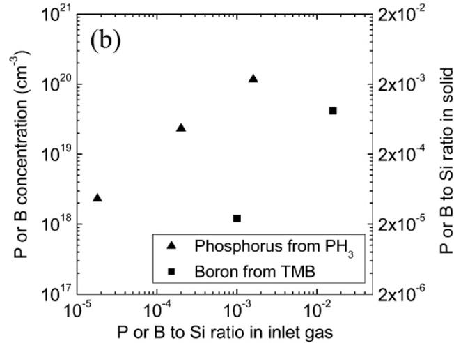
Figure 2.3. Phosphorus and boron concentration in silicon nanowires obtained by SIMS as a function of the dopant-to-silicon ratio in the gas phase. Taken from Wang et al.<sup>38</sup>
