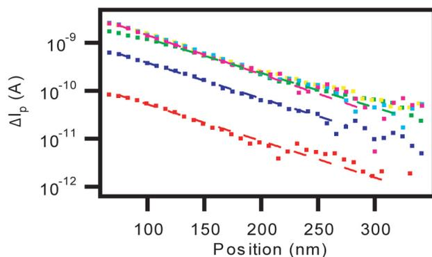
Figure 4.10. EBIC line profiles from an n-type silicon nanowire Schottky diode taken at different reverse bias voltages: Red 0 V, Blue 0.1 V, Green 0.3 V, Yellow 0.5 V, Cyan 1 V, Magenta 1.5 V. The dashed lines are exponential fits to the data (squares)
