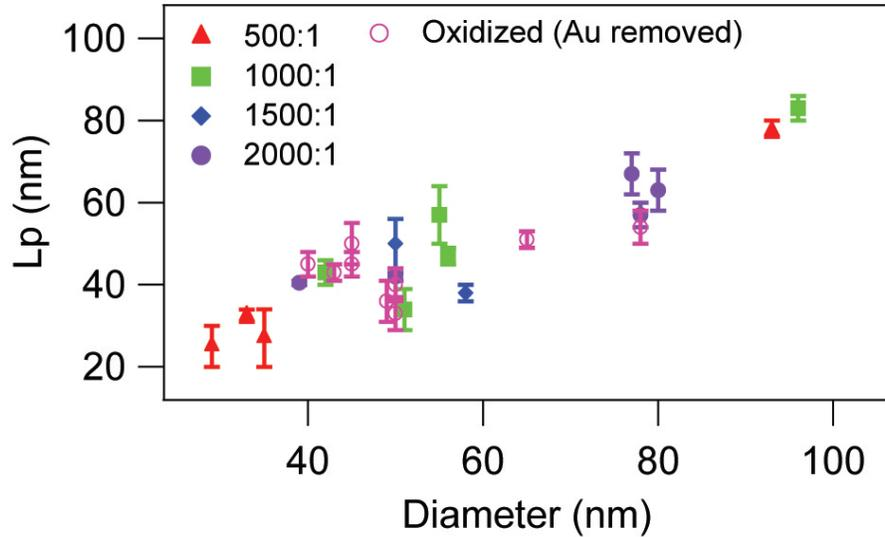
Figure 4.8. Plot of  $L_p$  versus diameter repeated from Figure 4.5 with the addition of results obtained from oxidized silicon nanowires. Diameter values for the oxidized wires are the core diameter determined from SEM images of the near-contact region.
