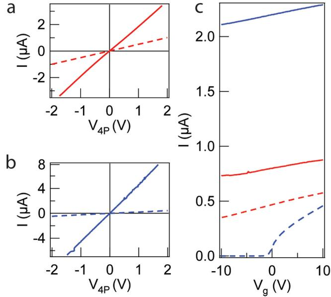
Figure 5.7. Change of nanowire conductivity with surface etching. (a),(b) Four-probe I-V data for devices before (solid line) and after (dashed line) etching of 2 nm and 4 nm, respectively. (c) Current versus gate voltage data for the devices in ‘c’ and ‘d’ showing n-type character and enhanced transconductance after etching.
