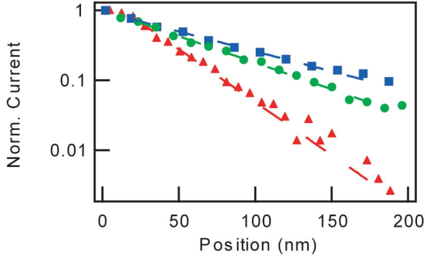
Figure 4.4. Semi-logarithmic plot of normalized EBIC profiles for nanowires having diameters of 93 nm (blue squares), 55 nm (green circles) and 35 nm (red triangles) with minority carrier diffusion lengths of 78 nm, 57 nm and 28 nm respectively. The dashed lines are exponential fits to the data.
