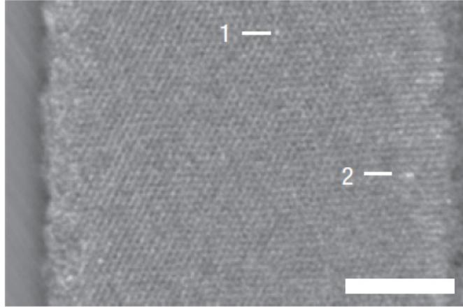
Figure 2.5. Abberation-corrected STEM image of gold atoms in a VLS-grown silicon nanowire. Scale bar is 5 nm. Taken from Allen and Hemesath et al.<sup>42</sup>
