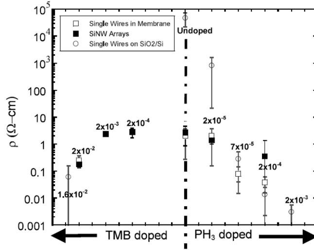
Figure 2.6. Plot of resistivity versus dopant-to-SiH<sub>4</sub> ratio for both phosphorous and boron doping. Taken from Eichfeld et al.<sup>46</sup>
