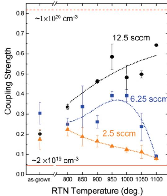
Figure 2.7. Fano resonance coupling strength versus annealing temperature for p-type silicon nanowires with different  $B_2H_6$  gas flow rates; 2.5 sccm (triangles), 6.25 sccm (squares), and 12.5 sccm (circles). The solid and dashed horizontal lines represent the coupling strength values obtained for boron-doped silicon wafers with doping levels of  $2 \times 10^{19}$  and  $1 \times 10^{20} \text{ cm}^{-3}$ , respectively. Taken from Eichfeld et al.<sup>56</sup>
