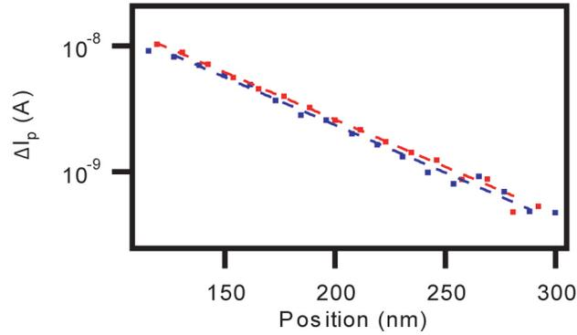
Figure 4.11. EBIC line profiles from an n-type silicon nanowire Schottky diode taken with different electron beam accelerating voltages. The dashed lines are exponential fits to the data (squares). The decay constant of the exponential does not change significantly between 5 kV (red) and 7 kV (blue) beams.
