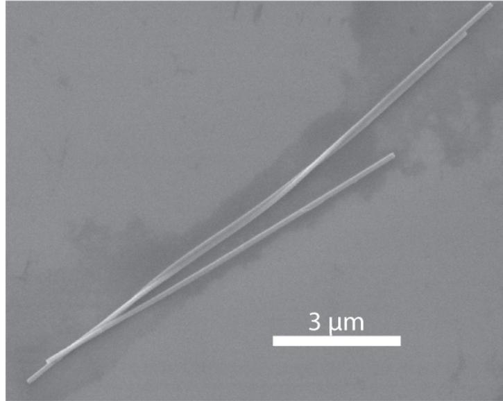
Figure 4.6. SEM image of silicon nanowires after removal of the gold catalysts.
