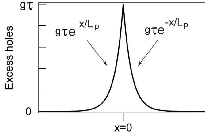
Figure 4.1. Calculated excess hole concentration vs position. Excitation at  $x = 0$  creates a steady state population of  $g\tau$  which decays exponentially with decay constant  $L_p$  when no external electric field is present.
