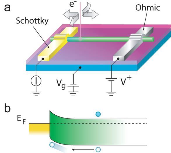
Figure 4.2. Schematic of EBIC measurement of a nanowire Schottky diode. (a) Diagram of a nanowire Schottky diode under reverse bias. (b) Band diagram showing excitation of excess carriers and diffusion of holes to the space-charge region.
