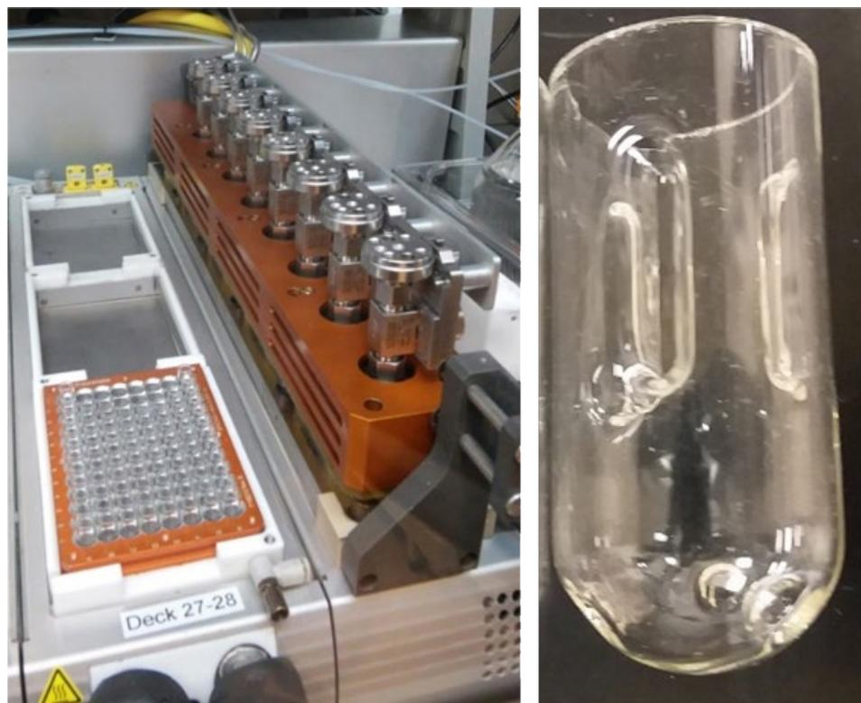
**Figure 4.7** Optimization Sampling Reactor (left) and vial with indentation (right).
