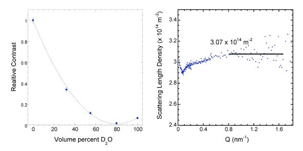
**Figure 5**: Contrast exchange parabola (left) and SLD value (right) for an alkali-activated slag (AAS) paste. See caption to Fig. 2 and text for more details. Note that the parabola at left has a minimum of zero intensity, indicating a single nanoscale phase in this paste (C-S-H).
