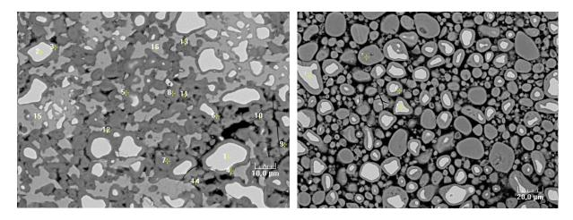
**Figure 6**: Backscattered electron micrographs (LCR). Left: Pure  $C_3S$  paste. Right:  $C_3S$  with colloidal silica, global CaO/SiO<sub>2</sub> ratio of 1.6. The measured Ca/Si ratio of the C-S-H gel in this paste is 1.2. This value is less than 1.6 because all of the colloidal SiO<sub>2</sub> has reacted but only 74% of the  $C_3S$ .
