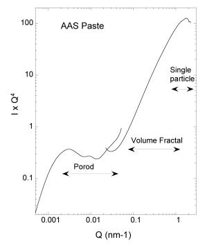
**Figure 4**: SANS data for alkali-activated slag paste mixed at w/s = 0.5 and hydrated for 3 months at 20°C. The data indicate a volume fractal regime corresponding to C-S-H at higher Q values and Porod scattering associated with the cores of unreacted slag particles at lower Q. The low-Q data was obtained using a different instrument (USANS).
