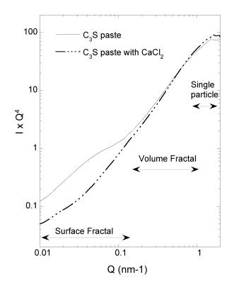
Figure 2: SANS data for C<sub>3</sub>S paste made with and without CaCl<sub>2</sub>.
