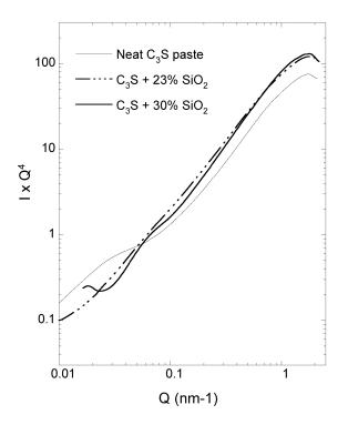
**Figure 7**: SANS data for  $C_3S$  pastes made with varying amounts of colloidal silica (See Table 1). For clarity, the SANS data for the paste with 40% SiO<sub>2</sub> is not shown, as it is very similar to that of the paste with 30% SiO<sub>2</sub>.
