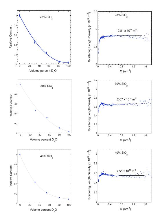
**Figure 8**: Contrast exchange curves (left) and SLD values (right) for  $C_3S + SiO_2$  pastes. See caption to Fig. 2 and text for more details.
