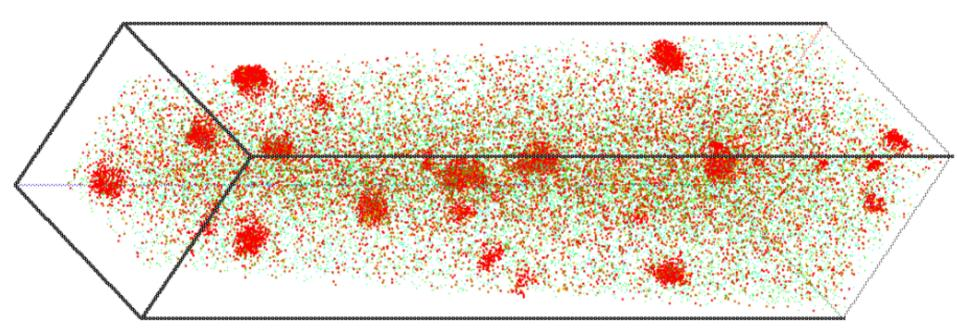
1,36 Cu, 0.85 Ni, 0.45 Mn steel, 0.06 C Solution treated and aged to maximum strength Red = Cu, Green = Ni. Fe not shown Box dimensions  $14 \times 14 \times 101$  nm<sup>3</sup>
