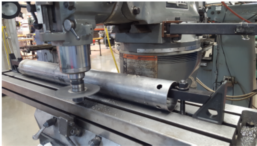
Figure 3.7. Longitudinal Cutting with Slitting Saw
