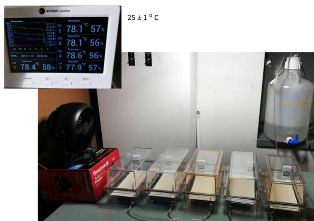
**Figure 3.2:** Setup of Aging Chamber
