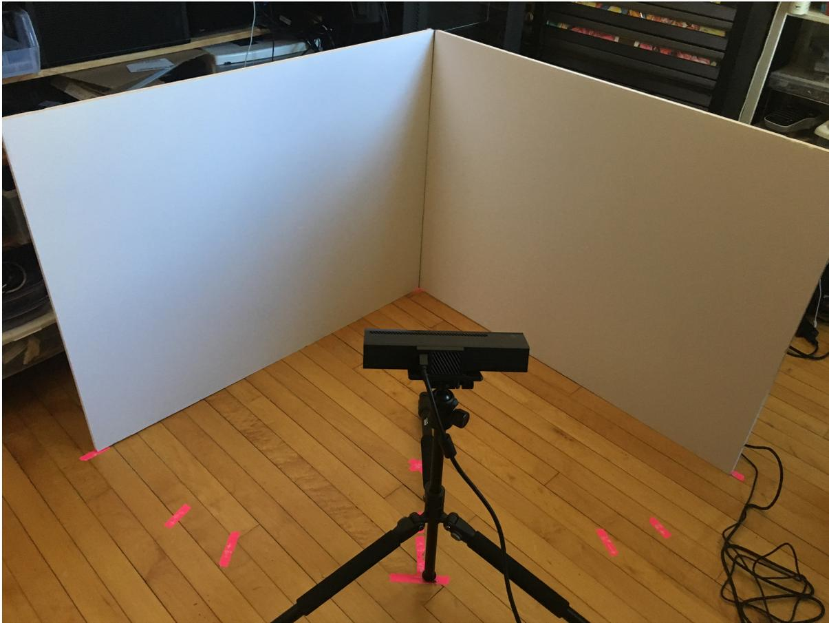
Figure 3.15. **Experimental Setup:** Foam core boards aligned to marks on the floor form a  $90^\circ$  v-groove. A Kinect ToF center is placed along the centerline and aligned with the center of the v-groove and the horizon. Kinect output was captured with a PC laptop. Board angles were then moved to  $60^\circ$  and  $45^\circ$  angles and captured with the Kinect.
