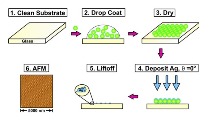
Figure 1. Fabrication of Ag nanoparticles via nanosphere lithography (NSL). (1) Glass substrate is cleaned. (2) Polystyrene nanosphere solution is drop-coated on to the glass. (3) Nanosphere solution is dried in ambient conditions. (4) Nanospheres form a hexagonally close-packed array. (5) Deposition of Ag onto nanospheres. (6) Removal of nanospheres by sonication. (7) AFM image of triangular Ag nanoparticles.
