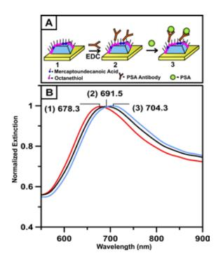
Figure 2: (A) A schematic representation of a PSA-antibody assay. (B) LSPR is the maximum extinction wavelength of the band,  $\lambda_{\text{max.}}$ , with extinction peak shifts in wavelength corresponding to the change in refractive index.
