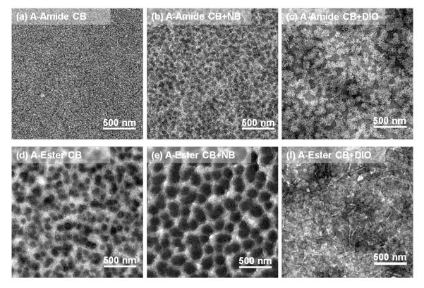
**Figure 4.14:** TEM images of donor/PC<sub>71</sub>BM blends cast either from single solvent (a,d) or from solvent mixtures (b,c,e,f).)
