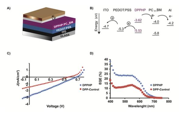
Figure 3.3: Schematic representation of the configuration of the solar cells fabricated (a). Energy diagram of all the components used in the devices described (b). Illuminated J – V curves of DPPHP and LDM (c). External quantum efficiency (EQE) spectra of DPPHP and LDM (d).
