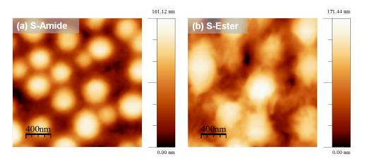
Figure 4.8: AFM topography images of solar cell morphology of (a) S-Amide/PC<sub>71</sub>BM and (b) S-Ester/PC<sub>71</sub>BM.
