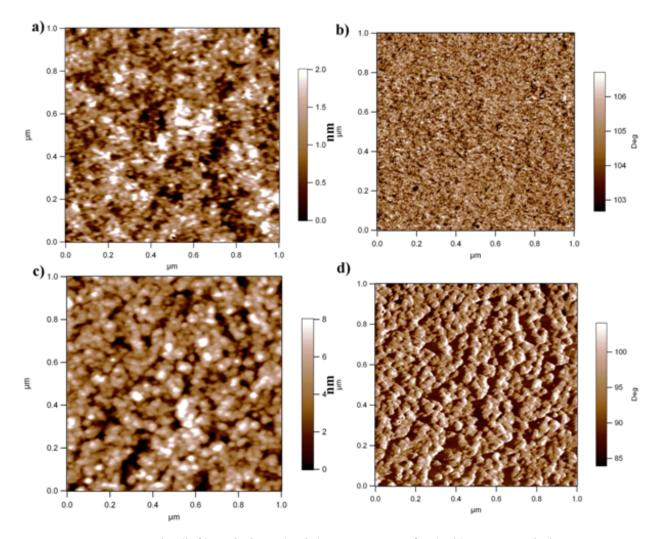
**Figure 1.23:** Topography (left) and phase (right) AFM images for (a, b) not annealed P3HT:PCBM (2000 rpm) and (c, d) annealed P3HT:PCBM (2000 pm). (reproduced from Ref.[90]
