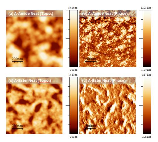
**Figure 4.17:** AFM topography (a,c) and phase (b,d) images of A-Amide and A-Ester neat films respectively, casted on mica from chlorobenzene and annealed at 100°C for 5 minutes.
