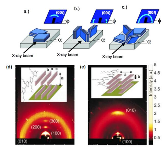
Figure 1.21: a) Schematic diagram showing the relationship between lamellar orientation and the resulting 2D-GIWAXS pattern: (a) lamellar structures oriented mostly parallel to the substrate surface; (b) lamellar structures oriented perpendicular to the substrate surface; (c) lamellar structures oriented randomly with respect to the substrate surface. (Ref.[86]) b) two different orientations of ordered P3HT domains with respect to SiO<sub>2</sub>/Si substrates (Reproduced from Ref.[85])
