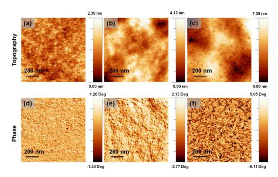
Figure 2.8: AFM topography and phase images of films created with the T<sub>C12</sub> donor. (a) and (d) are respectively the height and phase image of the material without any solvent additives, (b) and (e) with 0.8 volume percent DIO, and (c) and (f) contain both the same amount of DIO and 1.0 volume percent m-cresol.
