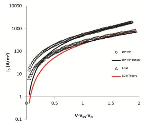
**Figure 3.15:** Experimental dark-current densities (J<sub>D</sub>) for DPPHP:PC<sub>71</sub>BM and LDM:PC<sub>71</sub>BM film blend devices at room temperature superimposed with curves calculated by the Child's law.
