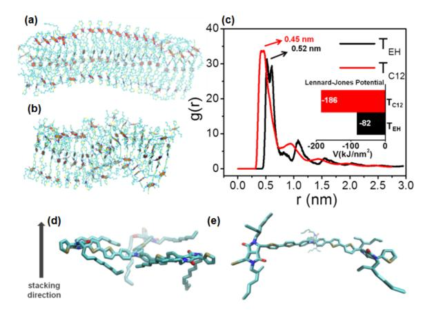
**Figure 2.6:** MD simulation of stacked (a)  $T_{C12}$  and (b)  $T_{EH}$  and (c) radial distribution function of the molecules with an inset of Lennard-Jones potential values. Single molecules from the MD stacking simulation for (d)  $T_{C12}$  and (e)  $T_{EH}$
