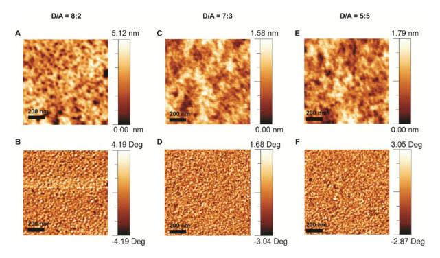
**Figure 3.9:** AFM of the active layers of DPPHP devices processed from chlorobenzene solutions at different donor/acceptor ratios (Height images in the top row, phase images in the bottom row).
