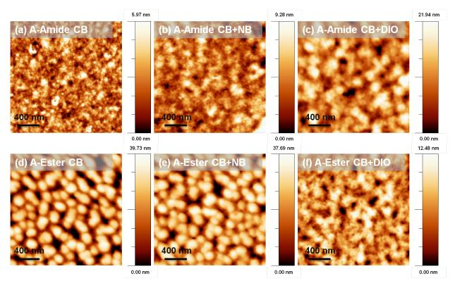
Figure 4.13: AFM images of donor/PC<sub>71</sub>BM blends cast either from single solvent (a,d) or from solvent mixtures (b,c,e,f).
