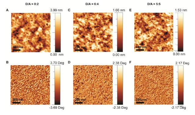
**Figure 3.10:** AFM of the active layers of DPPHP devices processed from toluene solutions at different donor/acceptor ratios (Height images in the top row, phase images in the bottom row).
