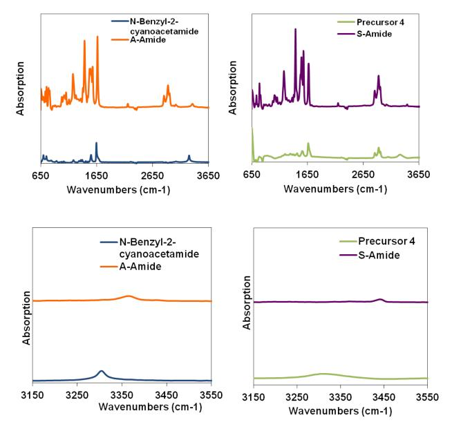
**Figure 4.6:** Infrared spectra of A-Amide with N-benzyl-2-cyanoacetate (left) and S-Amide with precursor 4 (right) with a close-up view of amide region (bottom).
