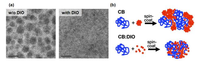
Figure 1.25: Examples of suppressing large-scaled phase segregation by solvent additives. (a) TEM images of PTB7/PC<sub>71</sub>BM BHJs (the scale bar is 200nm). (Reproduced from Ref.[17]) b) Schematics of PTB7/PC<sub>71</sub>BM blends in solution and thin-film states. (Reproduced from Ref.[97])
