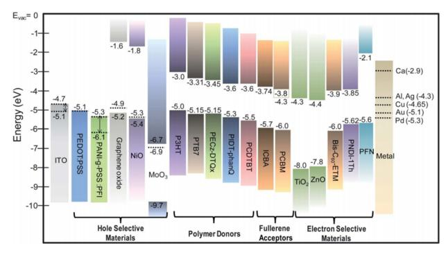
Figure 1.17: Schematic view of the energy gaps and energy levels of some of the components of recent OPVs including transparent electrodes, hole selective (transport) materials, polymer donors, fullerene acceptors, electron selective (transport) materials and metal electrodes. The dotted lines correspond to the work functions of the materials. Adapted from Ref.[55]
