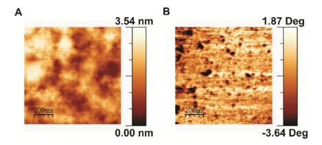
Figure 3.14: AFM height (a) and phase (b) images of the active layer of a LDM device. The LDM solution was prepared in toluene by the gradual cooling method and mildly mixed with  $PC_{71}BM$ . The scale bar is 200 nm in both images.
