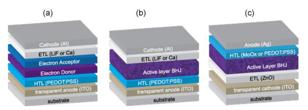
**Figure 1.5:** Schematics of common layers structures of OPVs in (a) bilayer normal geometry (b) BHJ normal geometry (c) BHJ inverted geometry (HTL=hole transport layer, ETL=electron transport layer).
