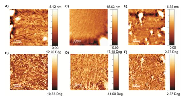
Figure 3.6: AFM height (top row) and phase images (bottom row) of thin films made by spin casting a solution of [DPPHP] =  $4.5 \times 10^{-3}$  M on mica. The scale bar is of 400 nm in all the images. Solution prepared by gradual cooling in chlorobenzene (a and b). Solution prepared by gradual cooling in toluene (c and d). Solution prepared by fast cooling in toluene (e and f).
