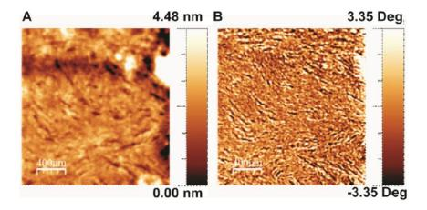
**Figure 3.11:** AFM height (a) and phase (b) images of a thin film spin cast from an assembled solution of DPPHP which was stirred for 12 hours. The fibers are shorter and less bundled. The scale bar is of 400 nm in both images.
