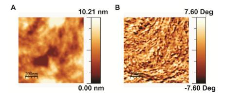
Figure 3.12: AFM height (a) and phase (b) images of a thin film spin cast from LDM in toluene. The solution was prepared by the gradual cooling method. The scale bar is 200 nm in both images.
