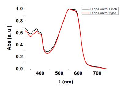
Figure 3.13: UV-vis spectra of fresh and aged LDM solutions in toluene. There are no signs of aggregation after aging.
