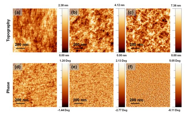
Figure 2.3: AFM topography images of  $T_{EH}$  cast from chloroform (a),  $T_{C_{12}}$  cast from chloroform (b), and  $T_{C_{12}}$  cast from chlorobenzene (c), with the corresponding phase images (d), (e), and (f), respectively.
