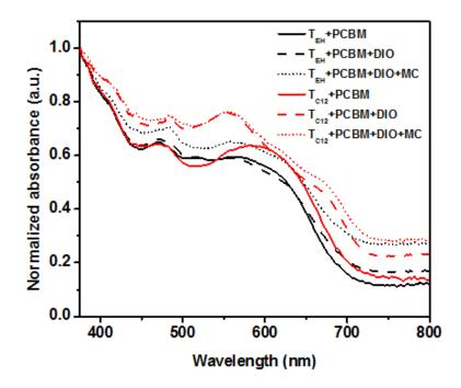
Figure 2.9: Absorption spectra of  $T_{EH}$  and  $T_{C_{12}}$  solar cells in solid film.
