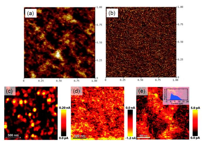
Figure 1.20: a) Tapping mode AFM topographic and phase images (1 mm 1 mm) of annealed films of pure P3HT (Ref.[83]) b)C-AFM Images taken on a P3HT/PC61BM solar cell after 2 min of annealing: electron-dominated dark current (collected at 5 V tip bias), hole-dominated dark current (collected at +5 V tip bias), and short-circuit photocurrent when excited with 532 nm laser light. Inset to right panel shows the photocurrent histogram. (Ref.[84])
