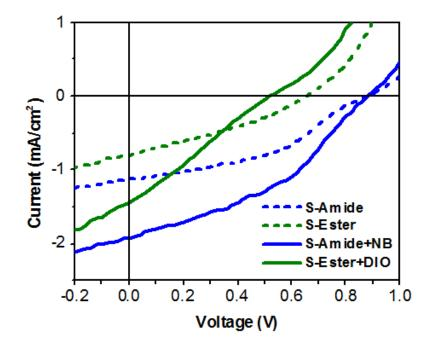
**Figure 4.9:** J-V characteristic of optimized solar cells of symmetric molecules with PC<sub>71</sub>BM under illumination
