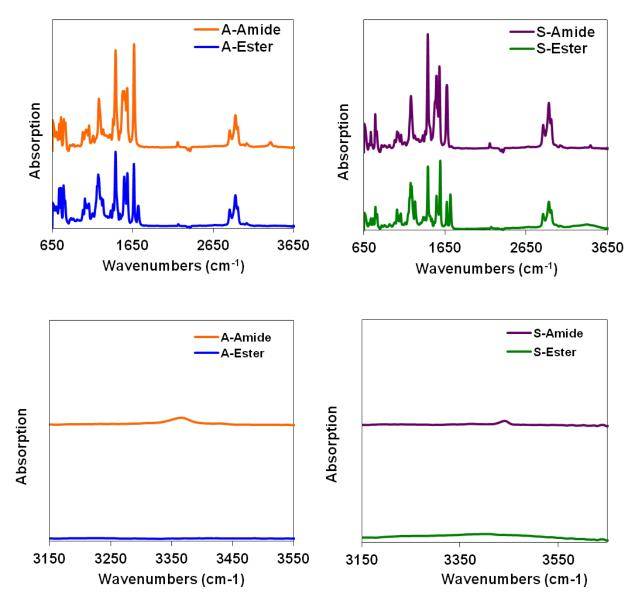
**Figure 4.5:** Infrared spectra of S-Amide and S-Ester (left) and A-Amide and A-Ester (right) with a close-up view of amide region (bottom).
