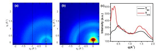
Figure 2.5: GIXD of  $T_{EH}$  (a) and  $T_{C12}$  (b) drop cast from chloroform. (c) Line profiles of GIXD data for  $T_{EH}$  and  $T_{C12}$ .
