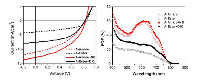
**Figure 4.10:** (a)J – V characteristics of optimized photovoltaic devices of asymmetric molecules with  $PC_{71}BM$  under illumination (AM 1.5). (b) EQE of the same devices.
