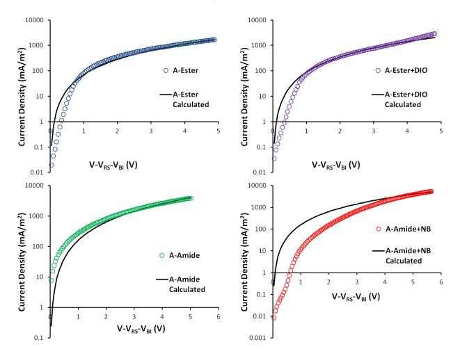
Figure 4.12: Experimental dark-current densities of A-Ester and A-Amide blends measured at room temperature in a hole only device configuration (empty marker). Experimental dark-current densities superimposed with curves calculated with SCLC theory (solid line)
