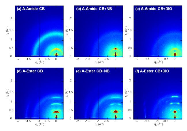
Figure 4.15: GIXD of donor/PC<sub>71</sub>BM blends cast from single solvent (a,d) or from solvent mixtures (b,c,e,f).
