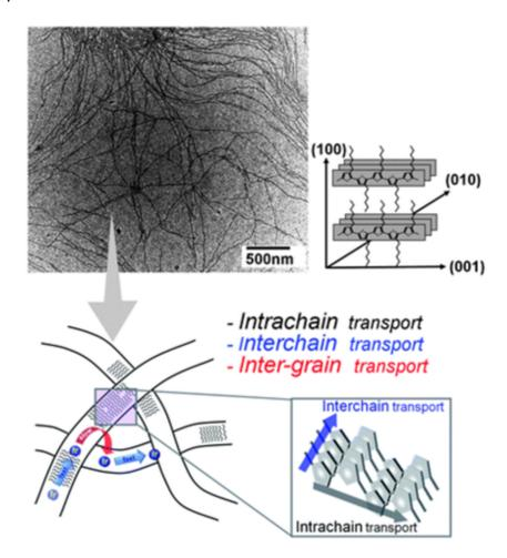
Figure 1.26: Schematic of the face-face stacking of polymer chains in P<sub>3</sub>HT nanowires. (Reproduced from Ref.[106])
