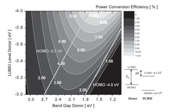
Figure 1.10: Contour plot showing the calculated energy-conversion efficiency (contour lines and colors) versus the bandgap and the LUMO level of the donor polymer according to the model described above. Straight lines starting at 2.7 eV and 1.8 eV indicate HOMO levels of – 5.7 eV and – 4.8 eV, respectively. A schematic energy diagram of a donor PCBM system with the bandgap energy (Eg) and the energy difference ( $\Delta E$ ) is also shown. Reproduced from Brabec et al.<sup>33</sup>
