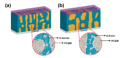
Figure 4.18: Schematic illustration of active layer morphology for A-Amide (a) and A-Ester devices (b).
