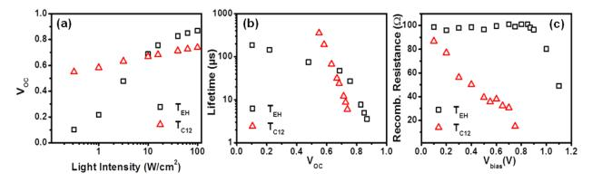
**Figure 2.13:** (a)  $V_{OC}$  versus light intensity, (b) lifetime versus  $V_{OC}$  (c) and recombination resistance versus applied bias (Vbias) of the optimized  $T_{EH}$  and  $T_{C12}$  devices.
