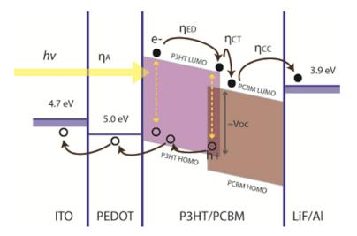
Figure 1.6: Illustration of OPV device operation with common materials.
