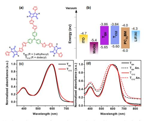
Figure 2.1: (a) Chemical structure of  $T_{EH}$  and  $T_{C12}$  molecules. (b) Energy levels of  $T_{EH}$  and  $T_{C12}$  molecules with the energy levels of other device layers. (c) Absorption spectra of  $T_{EH}$  and  $T_{C12}$  in chloroform solution and (d) in solid film cast from chloroform before and after annealing.
