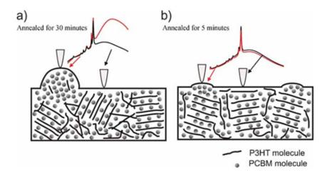
Figure 1.24: P3HT:PCBM blend films after a) 30-min. and b) 5-min. thermal annealing at 140°C. The red spectra were collected when the tip was positioned above the regions where PCBM aggregates were present. The black spectra were collected when the tip was away from the PCBM aggregates (Ref.[92]).
