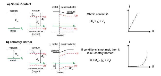
**Figure 1.16:** Energy levels for an Ohmic and a Schottky junction between a metal and a semiconductor. The current – voltage characteristics are shown schematically. Adapted from Ref.[54]
