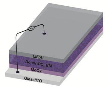
Figure 4.7: Schematic illustration of solar cell architecture used in this study
