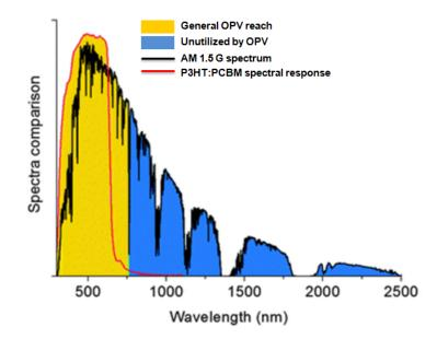
Figure 1.8: AM 1.5G spectrum and P3HT:PCBM spectral response, yellow band represents the reach of OPVs and blue band shows the non-utilized light. Take from Beliatis et al.<sup>31</sup>
