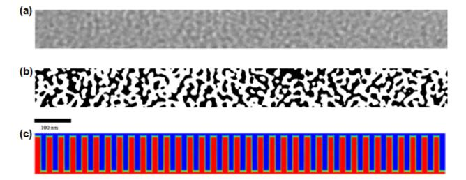
Figure 1.18: (a) Defocused ( $\Delta Z$ ) -25 µm) cross-sectional TEM images of the rrP3HT:PCBM BHJ active layer for 60 nm thinned slice, taken from Ref.[78] (b) Binary enhanced TEM image shown in (a) to be used as a guide to the eye. (c) Idealized BHJ active layer morphology showing interdigitated donor and acceptor with a width less than 20 nm, taken from Ref.[76].
