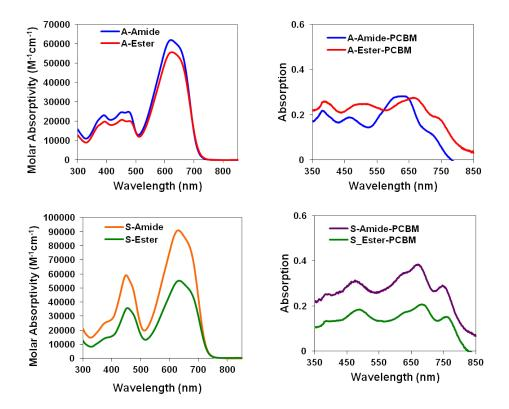
**Figure 4.3:** Absolute absorption of the four molecules in CHCl<sub>3</sub> (left) and unnormalized film absorption with PCBM under maximum PCE conditions (right).
