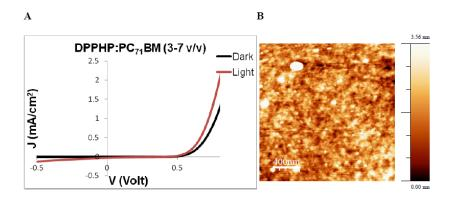
**Figure 3.4:** JV curve of devices fabricated by in situ self-assembly (a). Morphology of the active layer of devices fabricated by in single step self-assembly (b).
