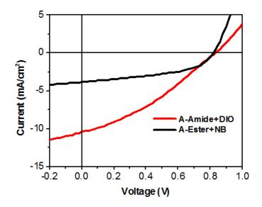
Figure 4.11: J-V characteristic of optimized solar cells of asymmetric molecules with different solvent additives under illumination.
