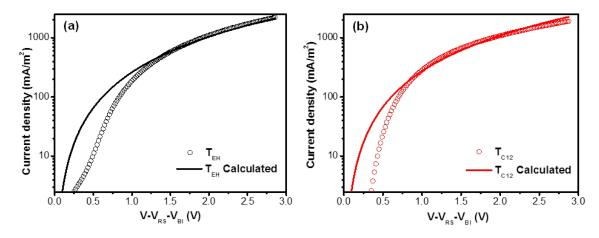
**Figure 2.12:** Experimental dark-current densities measured at room temperature in a hole-only device configuration (open circles) superimposed with curves calculated from SCLC theory (solid lines) for (a) T<sub>EH</sub>:PC<sub>71</sub>BM with DIO+MC and (b) T<sub>C12</sub>:PC<sub>71</sub>BM with DIO+MC.
