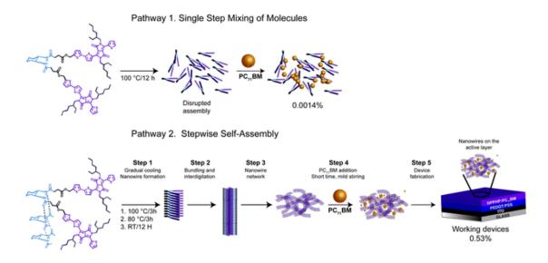
Figure 3.5: Schematic representation of the different preparation pathways used for device fabrication. Pathway 1 (top) shows the single step self-assembly of DPPPHP and  $PC_{71}BM$ . Route 2 (bottom) shows the stepwise self-assembly of DPPHP prior to the addition of  $PC_{71}BM$ .
