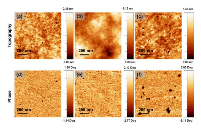
Figure 2.7: AFM topography and phase images of films created with the T<sub>EH</sub> donor. (a) and (d) are respectively the height and phase image of the material without any solvent additives, (b) and (e) with 0.8 volume percent DIO, and (c) and (f) contain both the same amount of DIO and 1.0 volume percent m-cresol.
