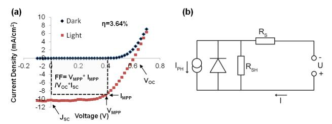
**Figure 1.7:** (a) Current density (J)- voltage (V) curve of a P<sub>3</sub>HT:PCBM standard device built in our lab. (b) equivalent circuit for a solar cell, described by the equation 2.
