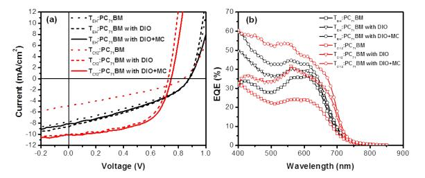
**Figure 2.11:** (a) J-V characteristics of optimized organic solar cells of tripod molecules with PC<sub>71</sub>BM under illumination (AM 1.5). (b) External quantum efficiency (EQE) of the same devices.
