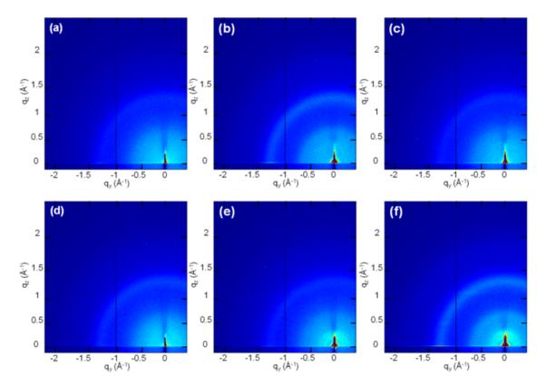
Figure 2.10: GIXD of  $T_{EH}$ :PC<sub>71</sub>BM blend casted from chloroform (a), chloroform + DIO (0.8% v/v) (b) and chloroform + DIO (0.8% v/v) + MC (1% v/v) (c);  $T_{C12}$ :PC<sub>71</sub>BM casted from chloroform (d), chloroform + DIO (0.8% v/v) (e) and chloroform + DIO (0.8% v/v) + MC (1% v/v) (f).
