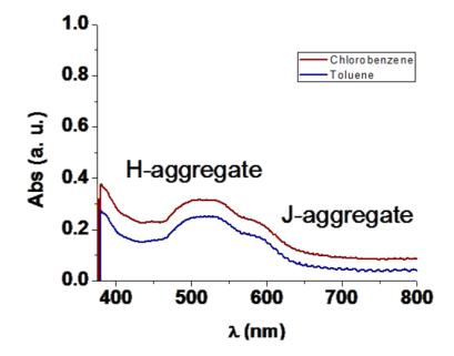
Figure 3.8: Absorption spectra of DPPHP thin films spin cast on mica at 1500 rpm in toluene and chlorobenzene.  $[DPPHP] = 4.5 \times 10^{-3} M$
