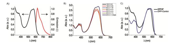
Figure 3.2: Normalized absorption and emission spectra ( $\lambda ex = 573$  nm) of DPPHP in chlorobenzene. [DPPHP] =  $4.5 \times 10^{-3}$  M. [DPPHP] =  $0.27 \times 10^{-3}$  M for emission measurements (a). Absorption spectra of DPPHP in toluene at different temperatures. [DPPHP] =  $4.5 \times 10^{-3}$  M (b). Normalized absorption spectra of DPPHP and LDM in toluene. [DPPHP] =  $4.5 \times 10^{-3}$  M, [LDM] =  $1.2 \times 10^{-3}$  M (c).
