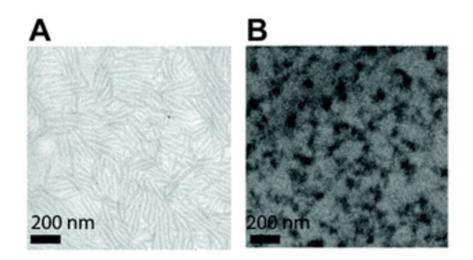
Figure 3.7: Cryo-TEM image of a DPPHP solution in toluene prepared following the stepwise self-assembly pathway. [DPPHP] = 7 mg ml<sup>-1</sup> (a). Cryo-TEM image of a DPPHP:PC<sub>71</sub>BM blend in a 1:1 ratio mixed for 30 seconds. [DPPHP] = 7 mg ml<sup>-1</sup> and [PC<sub>71</sub>BM] = 27 mg ml<sup>-1</sup> (b).
