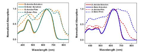
Figure 4.2: Absorption spectra of symmetric and asymmetric donors in CHCl<sub>3</sub> and on film.
