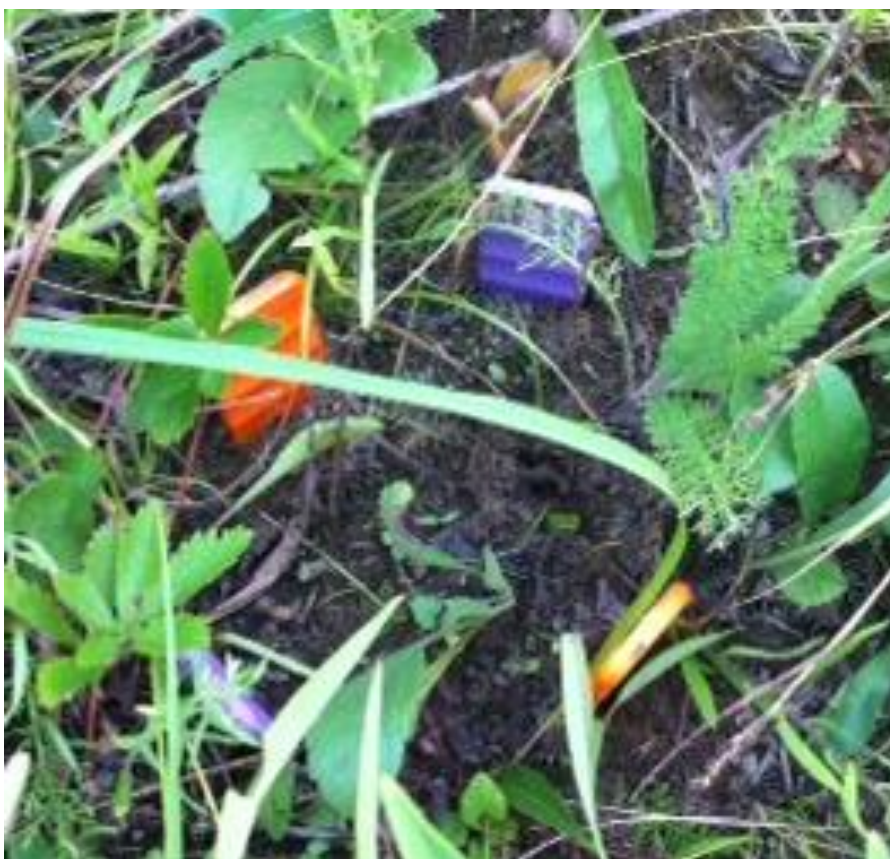
Ch1. Figure 4: PRS probe arrangement. Two sets of two cation (purple) and two anion (orange) probes were installed 5 m from the center point of each plot.
