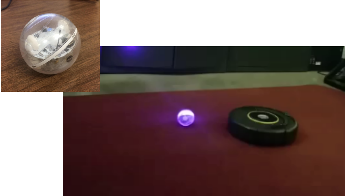
Figure 9.5. The sphero SPRK robot and the experiment setup (the Roomba robot is used only as the object of estimation). The sphero SPRK internal mechanism shifts the center of mass by rolling and rotating within the spherical enclosure. RGB LEDs on the top of the sphero SPRK are utilized to track the odometry using a Microsoft Kinect. The robot is equipped with a collision detection feature that we use to acquire binary (collision/no-collision) measurements in real time. The Robot Operating System (ROS, available online [13]) is used to transmit and collect data at 20 Hz.
