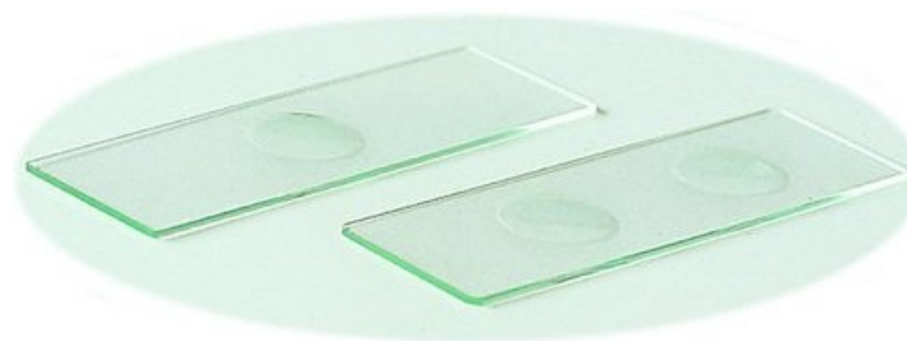
Figure 4.9. Glass slides with either one or two spherical depressions (16 mm diameter; 0.50 mm depth) for holding liquid samples.
